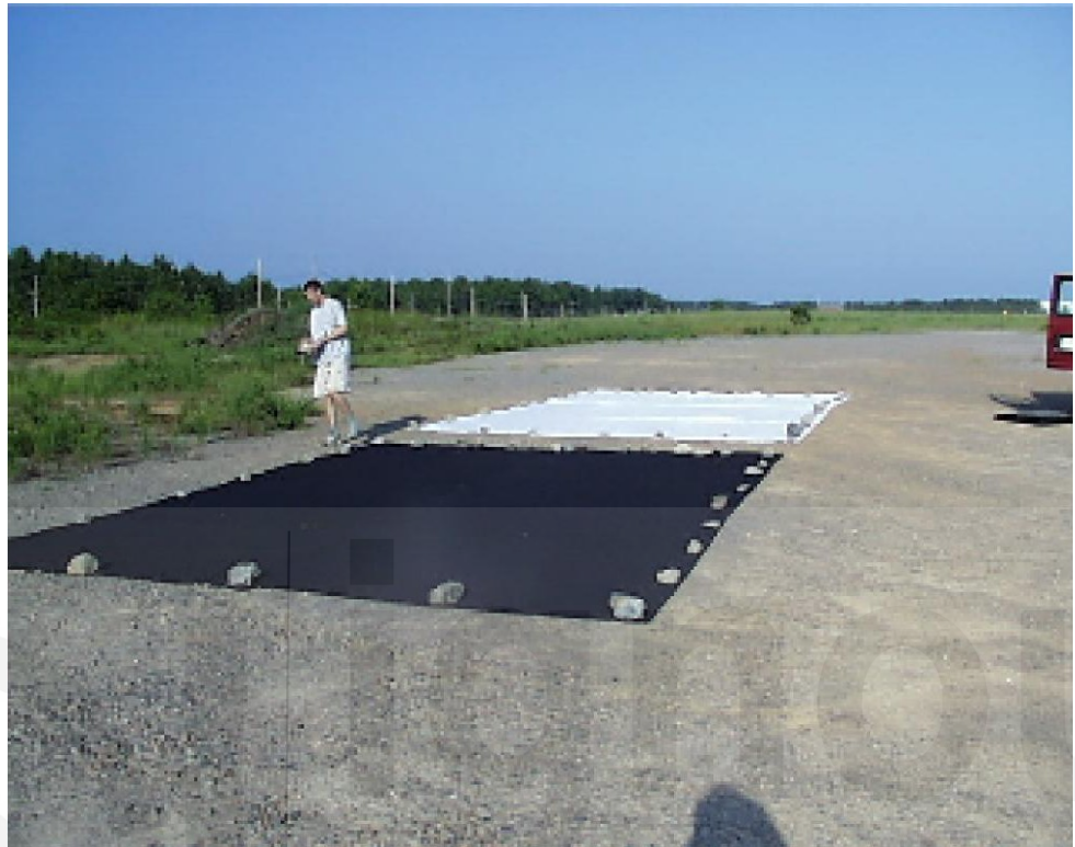
Fig. 8.6: Preparation of test sites for calibration purposes. (Source: Lecture slides of Prof. J.R. Jensen, University of South Carolina; used with permission)
