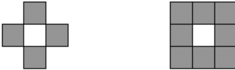
Fig. 15.7: Two definitions of a raster cell's neighbourhood. In the rook's case only the four cells that share an edge are neighbours, but in the queen's case the neighbourhood includes the four diagonal neighbours.
