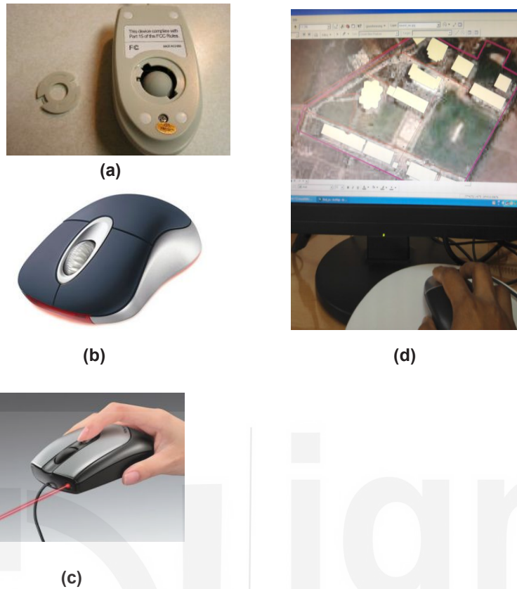
Fig. 8.4: Mouse and digitisation: a) Rollar ball; b) Optical mouse; c) Laser mouse; and d) On-screen digitisation with the help of mouse.
