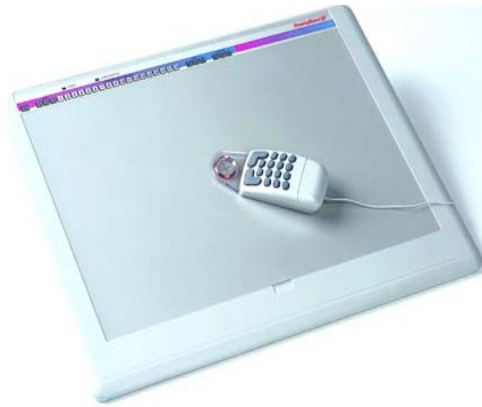
Fig. 8.3: Digitising table and puck. (Source: http://proceedings.esri.com/library/userconf/proc01/professional/papers/pap894/p894.html )
