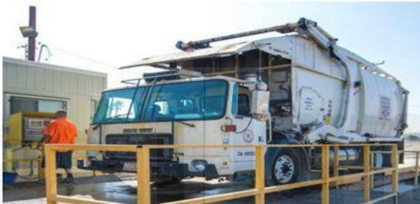
Figure 5.1: Weighing of collection vehicle (truck)
