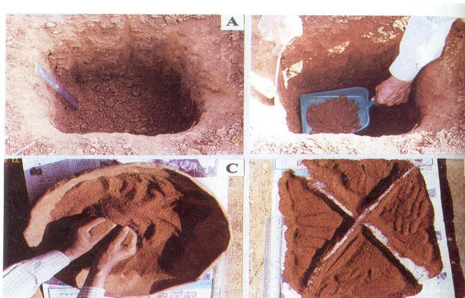
Fig.1.1: Process of collection of soil samples
