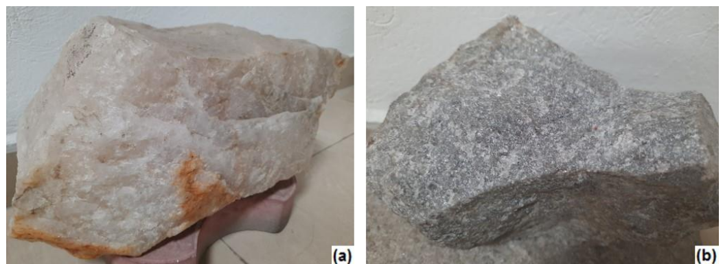
Fig. 15.10: Quartzite samples from IGNOU Headquarters: a) Quartzose quartzite; and b) Ferruginous quartzite.
