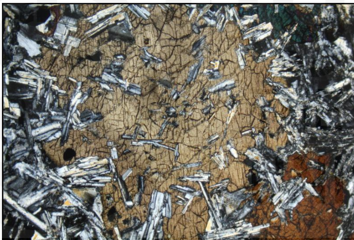
Fig. 14.1: Photomicrograph showing plagioclase laths, as inclusion within big augite crystal indicative of blasto-ophitic texture, under XP. Note few plagioclase laths on the margin are partially enclosed. (Field of View = 2mm; Source: www.alexstrekeisen.it )
