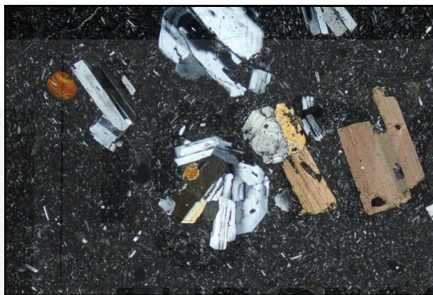
Fig. 14.3: Photomicrograph showing larger crystals of plagioclase, biotite and clinopyroxene clustered and surrounded by fine grained groundmass depicting blasto-porphyritic texture. (Source: www.alexstrekeisen.it )
