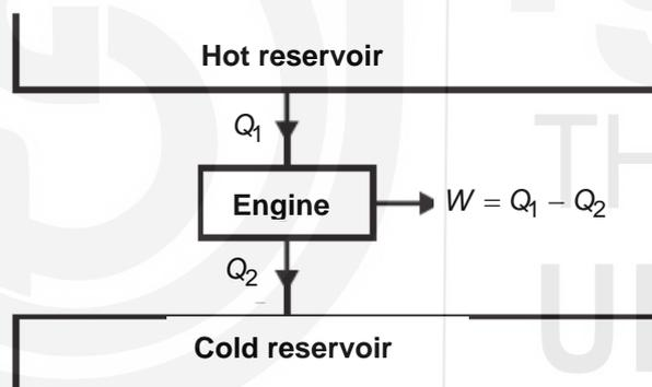
Fig. 8.1: Schematics of operation of a heat engine.
