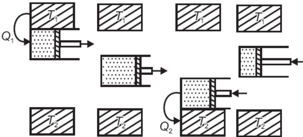
Fig. 8.2: Four stages in the Carnot cycle.
