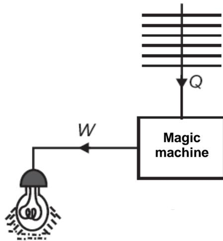
Fig. 8.7: Illustrating the proof of Carnot's theorem.
