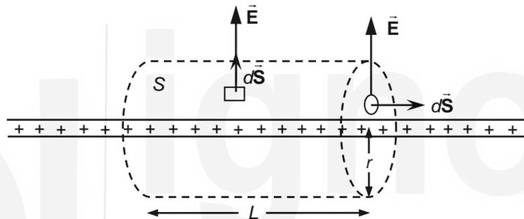
**Fig. 7.5: Applying Gauss's law to an infinite uniformly charged wire carrying positive charge. The Gaussian surface is cylindrical having length  $L$  and radius  $r$ . It encloses a section of the charged wire.**
