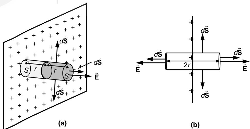
Fig. 7.9: a) A sheet of positive charge and the Gaussian pillbox for which the electric field  $\vec{E}$  and area vector  $d\vec{S}$  are parallel at the ends and perpendicular to each other on the curved part of the surface; b) the sheet in its side view showing the electric field vectors and area vectors for the pillbox.
