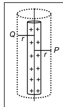
**Fig. 7.3: The magnitude of the electric field due to a cylindrical charge distribution at any point depends on its perpendicular distance  $r$  from the axis of symmetry. If it were not so, the magnitude of the electric field would be different at different points, (e.g.,  $P$  and  $Q$ ) on the same surface for the same charge distribution, which is incorrect.**
