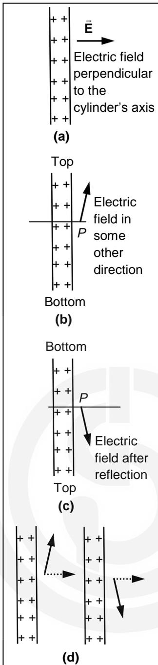
**Fig. 7.2:** a) The direction of electric field  $\vec{E}$  due to a section of an infinite charged cylinder is perpendicular to its axis; b) electric field in some other direction; c) reflected electric field; d) the directions of electric fields are different at the same point for the same charge distribution, which is not possible. So,  $\vec{E}$  can only be in the direction shown by dotted arrows.
