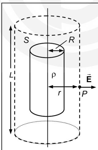
**Fig. 7.6: Electric field at a point  $P$  lying outside a uniformly charged infinite cylinder. The cylindrical Gaussian surface is of length  $L$  and radius  $r > R$ .**
