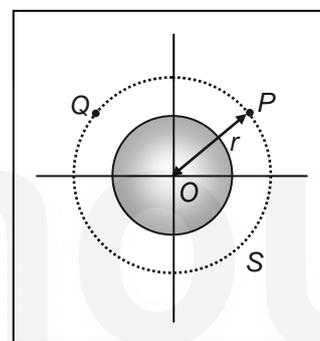
**Fig. 6.10:** The magnitude of the electric field at any point  $P$  on the spherical surface  $S$  depends only on the radius  $r$  of the surface, i.e., the radial coordinate of  $P$ . Due to spherical symmetry, it is independent of the angular coordinates of the point.
