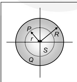
**Fig. 6.13: Determining the electric field of a uniformly charged sphere of radius  $R$  carrying net charge  $Q$  at a point  $P$  inside the sphere.**
