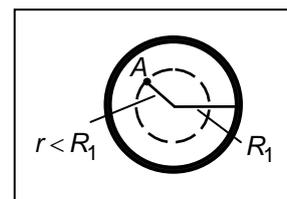
Fig. 6.18: The electric field at a point inside the inner shell is zero since the charge enclosed by it is zero.
