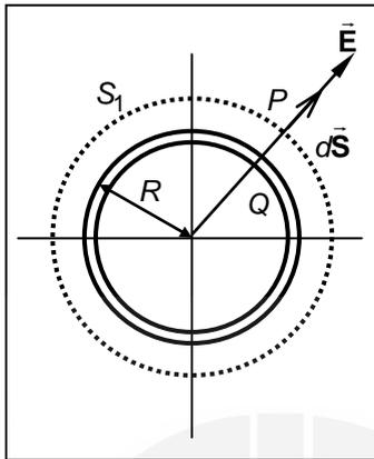
**Fig. 6.15:** A thin uniformly charged spherical shell of radius  $R$  carrying a net charge  $Q$ . The cross-section of the Gaussian surface  $S_1$  is shown for a point lying outside the shell. It is concentric with the shell.
