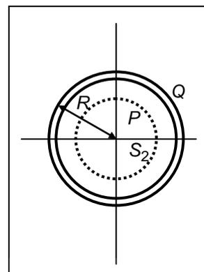
Fig. 6.16: The cross-section of a Gaussian surface  $S_2$  enclosing the empty interior of the thin uniformly charged spherical shell of radius  $R$  carrying a net charge  $Q$ .
