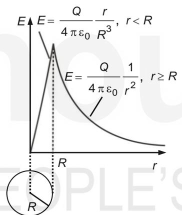
**Fig. 6.14:** The behaviour of the electric field due to a uniformly charged sphere of radius  $R$ .
