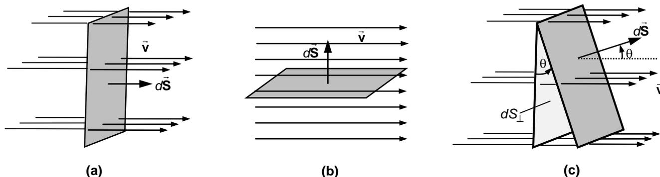
Fig. 6.1: A wire loop placed in a stream a) normal and b) parallel to the direction of the flow or the velocity field  $\vec{v}$ ; c) the same loop placed at an angle  $\theta$  to the direction of fluid flow. In parts (a) and (c) of this figure, we have shown only a few lines for the fluid flow but the loop is immersed in the stream.
