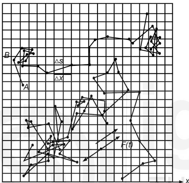
Fig. 4.4: Calculation of  $\overline{x^2}$  for a Brownian particle.
