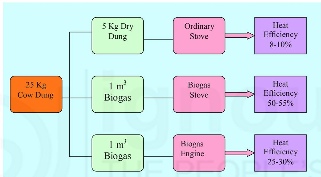
Figure 4.6 : Efficiency of Energy Conversion of Dung
