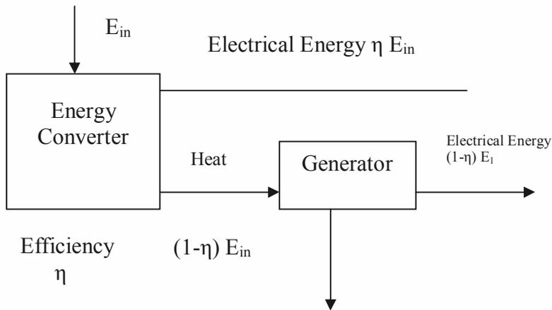
Figure 4.2 : Energy Conversion with Rejected Heat
