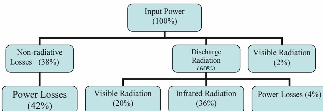
**Figure 4.5 : Energy Distribution in a Fluorescent Lamp**
