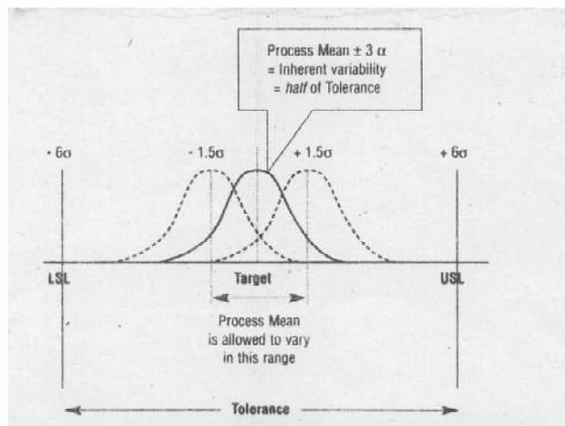
Fig. 3.8: The Six Sigma Process:  $USL = \text{Mean} + 3 \text{ sigma}$ ,  $LSL = \text{Mean} - 3 \text{ sigma}$
