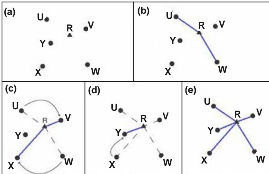
Fig. 3.2: Steps describing the Rapid Static measuring technique; (a) describes Step 1, (b) describes Step 2, (c) describes Step 3, (d) describes Step 4 and (e) describes Step 5 (source: modified from Leica Geosystems AG, 1999)
