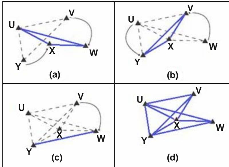
Fig. 3.1: Steps describing the Static measuring technique; (a) describes Step 1, (b) describes Step 2, (c) describes Step 3 and (d) describes Step 4 (source: modified from Leica Geosystems AG, 1999)
