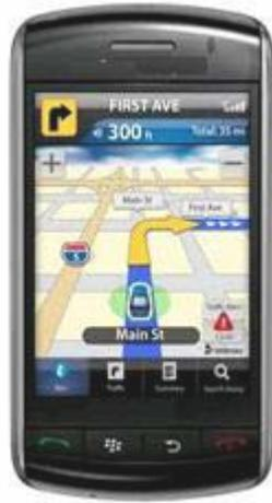
Fig. 2.3: A handheld GPS receiver
