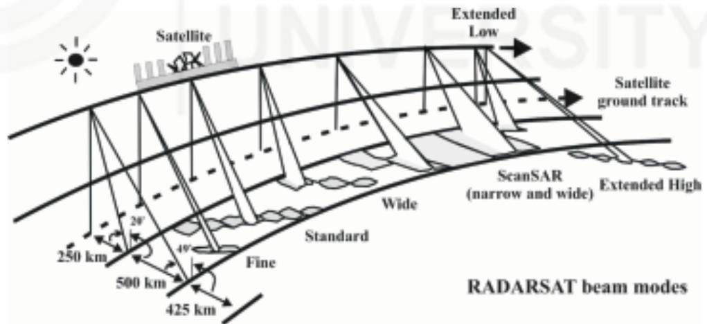
Fig. 6.11: RADARSAT-1 imaging modes (source: www.asc-csa.gc.ca)
