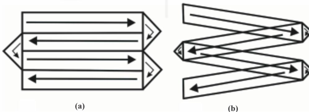
Fig. 6.9: (a) Scan line corrector mode of Landsat-7 and (b) failure of SLC (source: [www.landsat.usgs.gov](http://www.landsat.usgs.gov))
