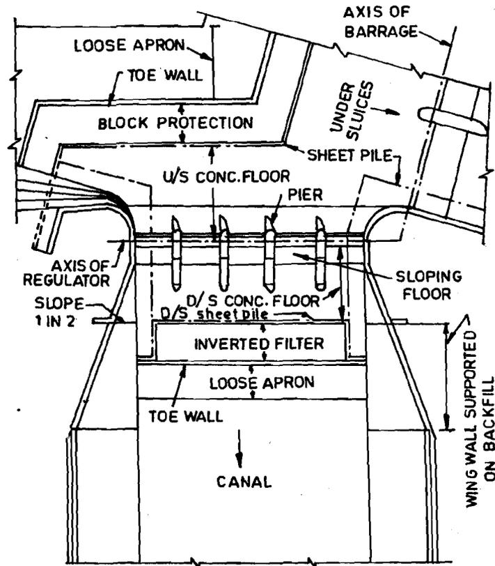
Figure 13.1 : Plan of a Canal Head Regulator
