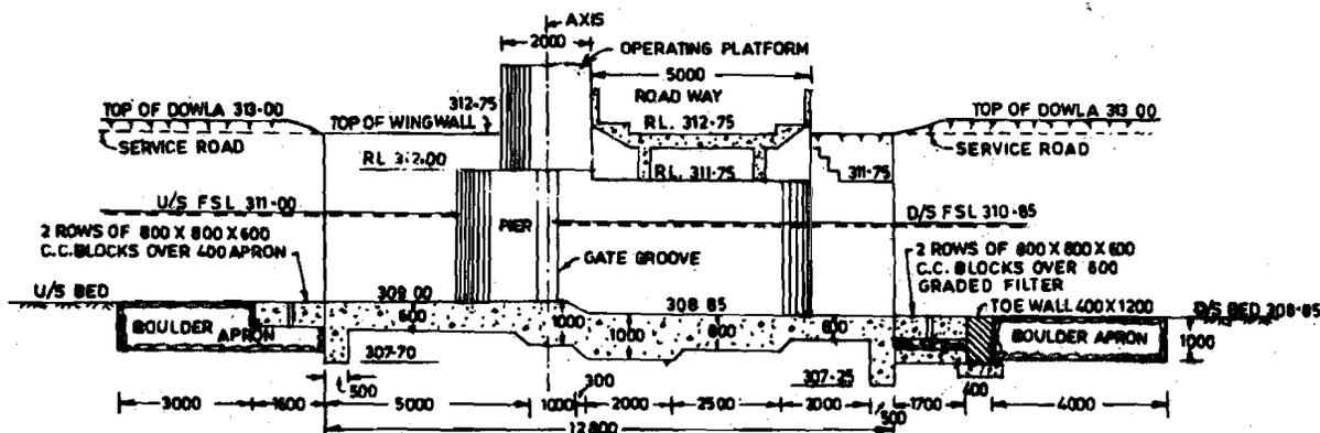
Figure 13.5 : Section at A-A through a Cross Regulator (See Figure 13.3)
