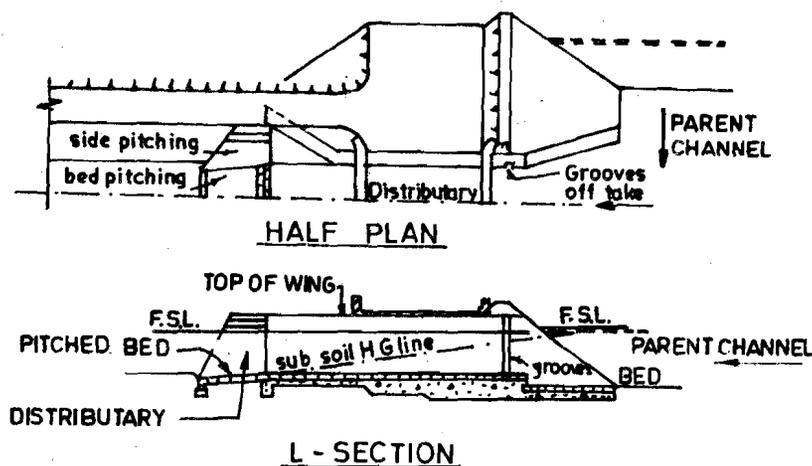
Figure 13.6 : Simple Distributary Head Regulator
