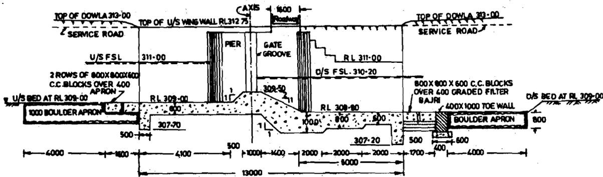
Figure 13.4 : Section at B-B through Distributary Head Regulator (See Figure 13.3)
