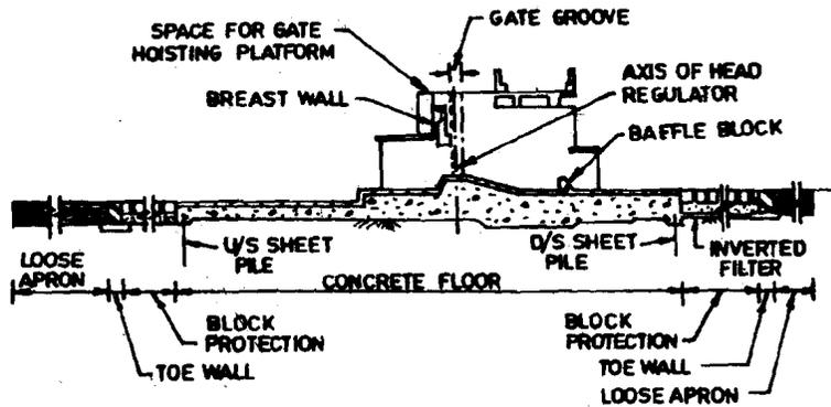
Figure 13.2 : Section of Canal Head Regulator
