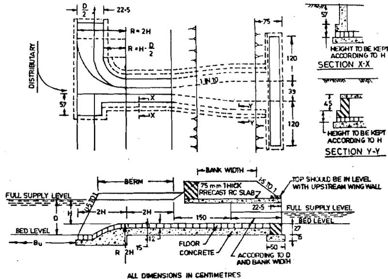
Figure 10.3 : Plan of Open Flume Outlet (For Distributary above 0.6 m Depth and H less Full Supply Depth)
