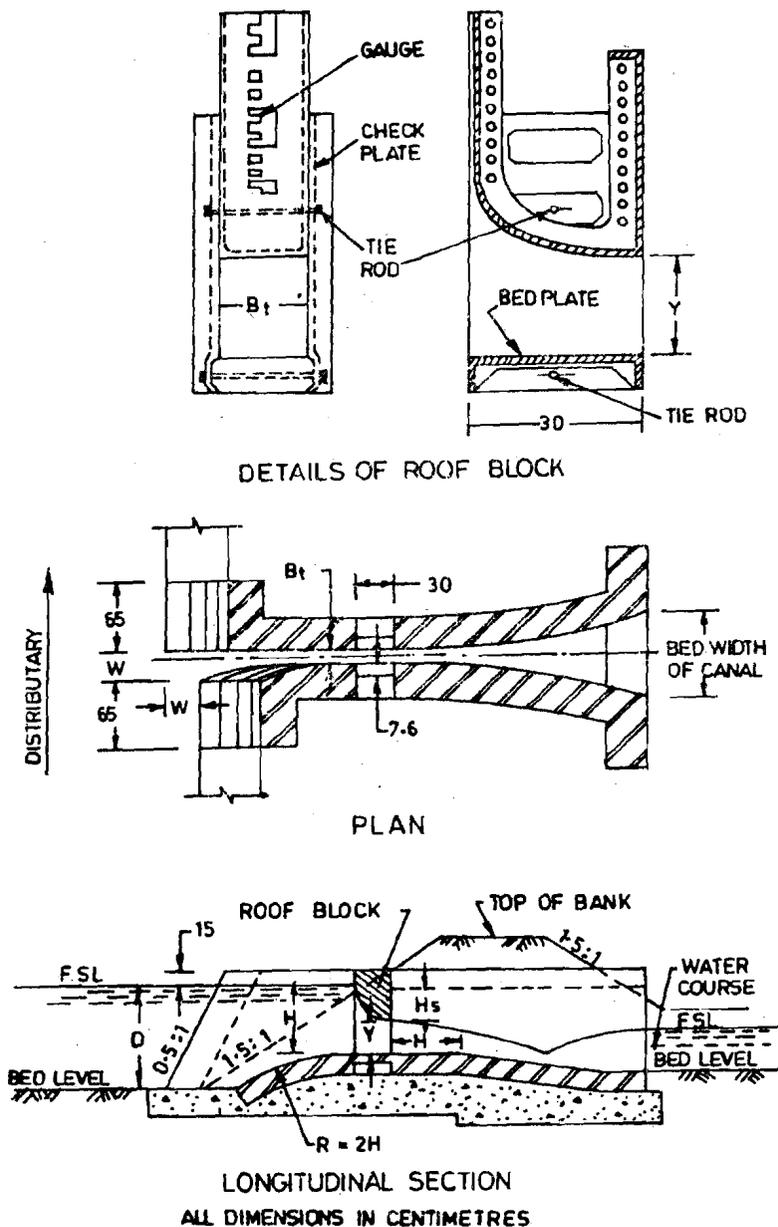
Figure 10.4 : Crump's Adjustable Module
