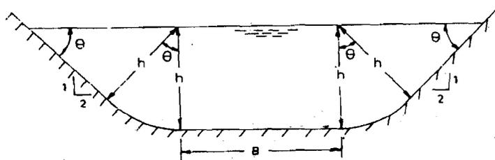
Figure 9.11 : Lined Channel Section for  $Q > 55 \text{ m}^3/\text{s}$
