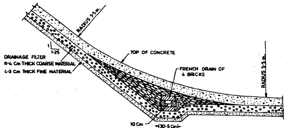
Figure 9.12 : A Typical Drainage Arrangement behind a Lining
