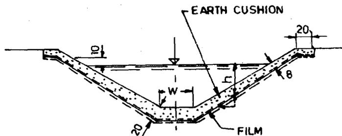
Figure 9.8 : Canal Lining with PVC Film
