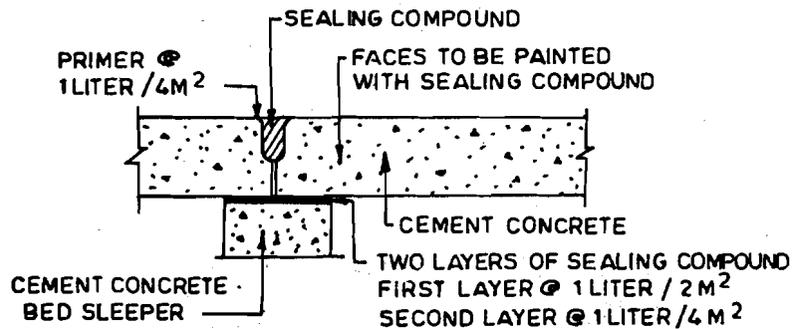
Figure 9.2 : Details of Construction Joints
