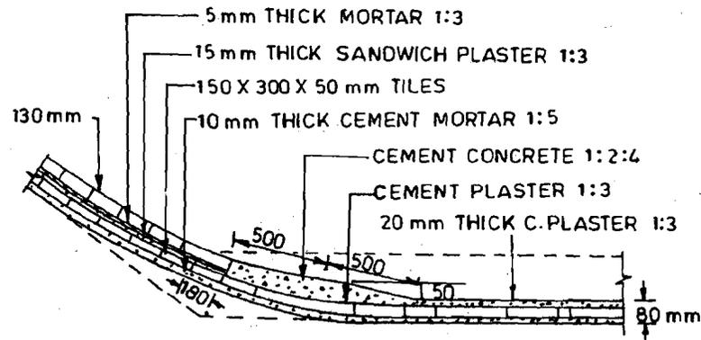
Figure 9.6 : Double Tile Lining on Banks, and Single Tile Lining on Bed
