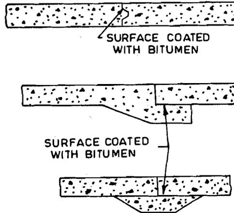
Figure 9.1 : Joints in Concrete Lining
