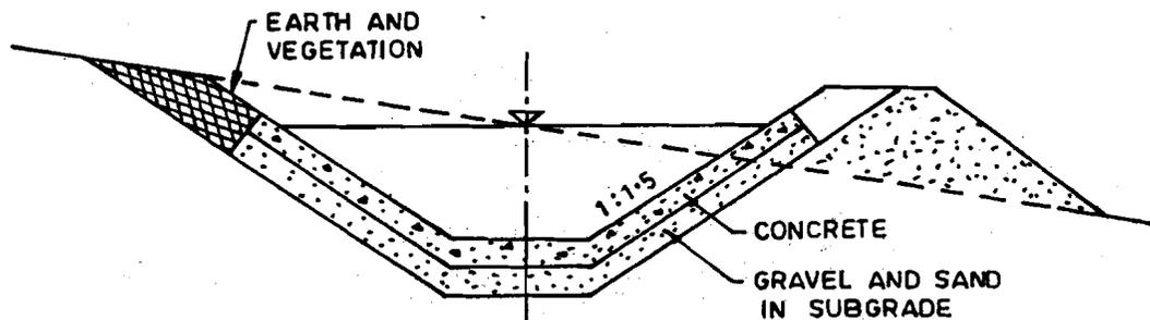
Figure 9.3 : Two-layer Lining of Monolithic Concrete
