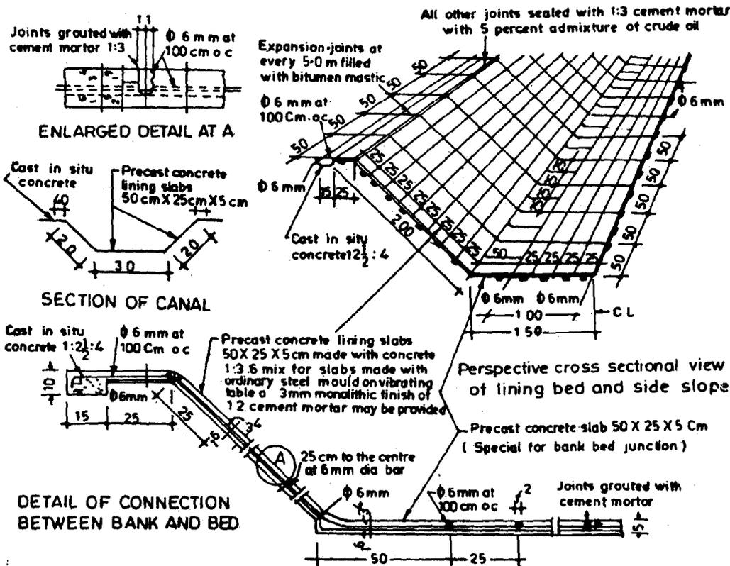
Figure 9.5 : Details of Precast Concrete Lining
