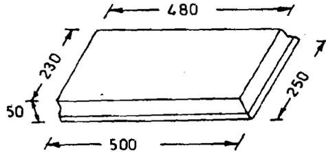
Figure 9.4 : Details of Pre-cast Slab
