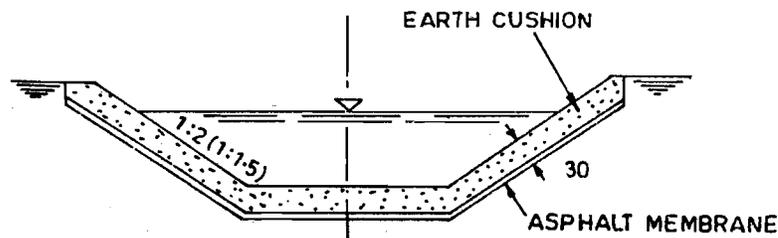
Figure 9.7 : Cross-Section of Canal Sealed by an Asphalt Membrane
