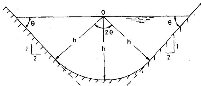
Figure 9.10 : Lined Channel Section for  $Q < 55 \text{ m}^3/\text{s}$
