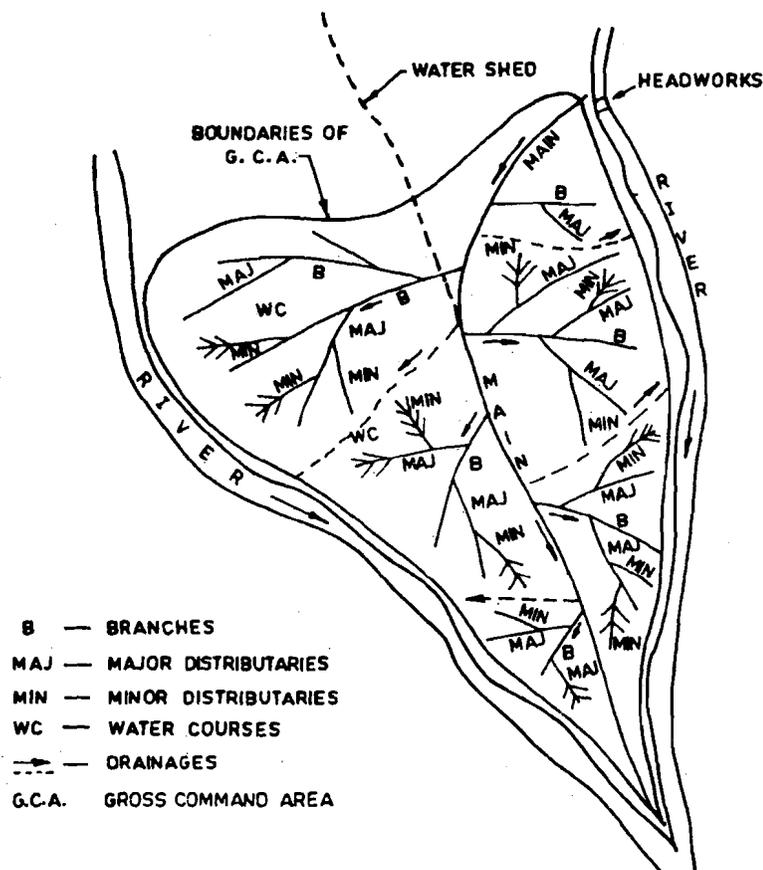
Figure 7.2 : Schematic Layout of a Canal Distribution System
