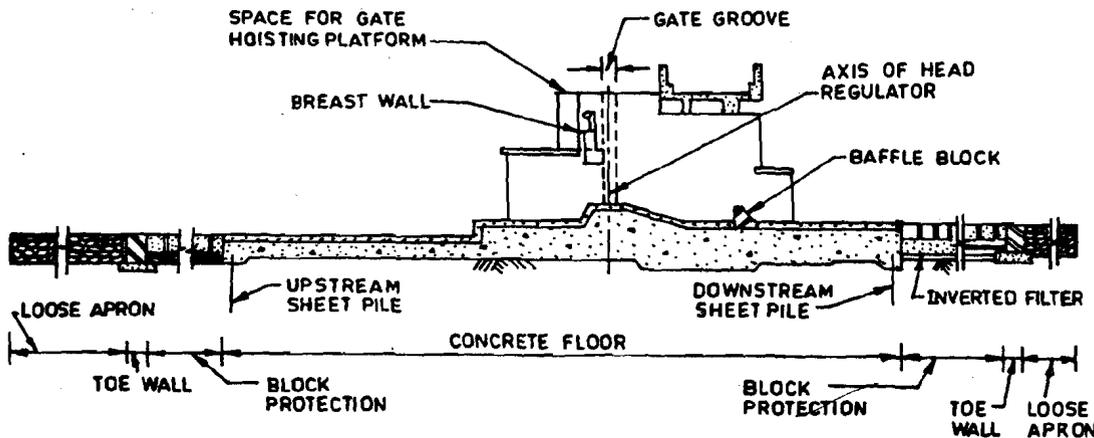
Figure 5.2 : Cross-section through a Head Regulator
