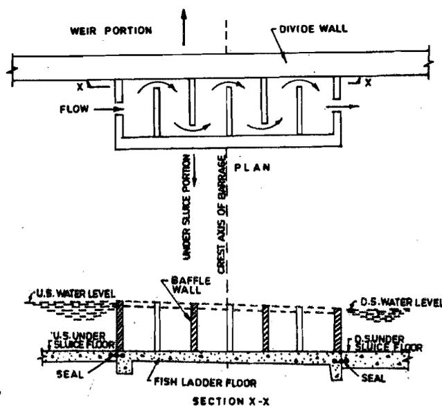
Figure 5.4 : Typical Cross-section of a Fishway
