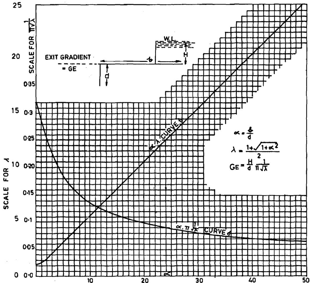
Figure 5.8 : Khosla's Curve for Exit Gradient
