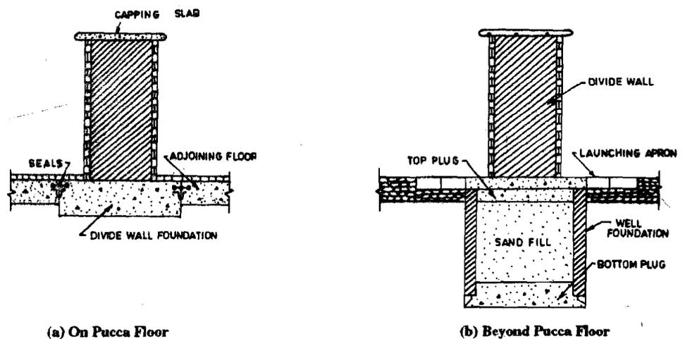
Figure 5.3 : Cross-section of Divide Wall
