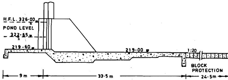
Figure 4.4 : Cross-section through a Barrage
