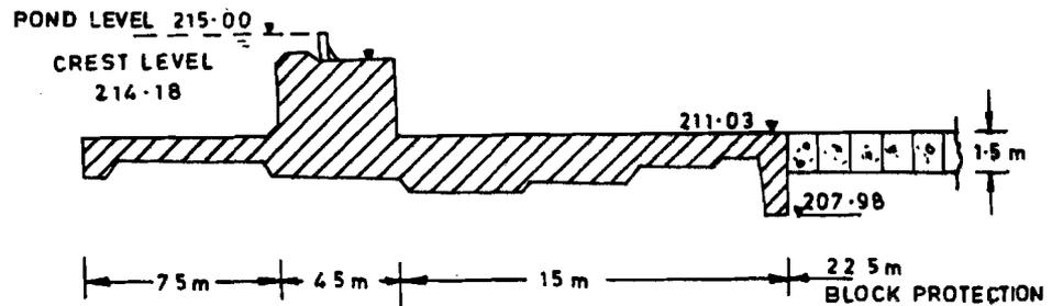
Figure 4.1 : Masonry Weir
