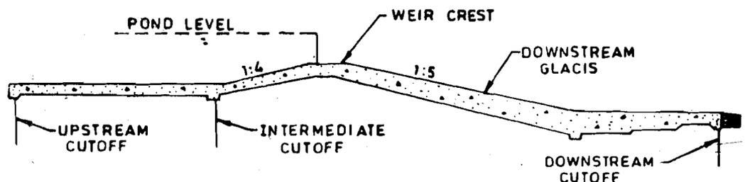
Figure 4.3 : Concrete Weir
