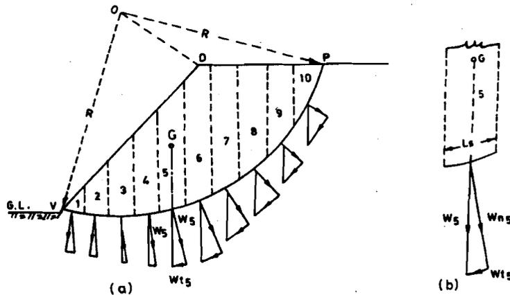
Figure 3.7 : Swedish Method for C -  $\phi$  Soil
