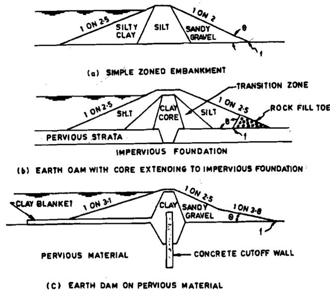
Figure 3.1 : Cross-sections of Typical Earth Dams
