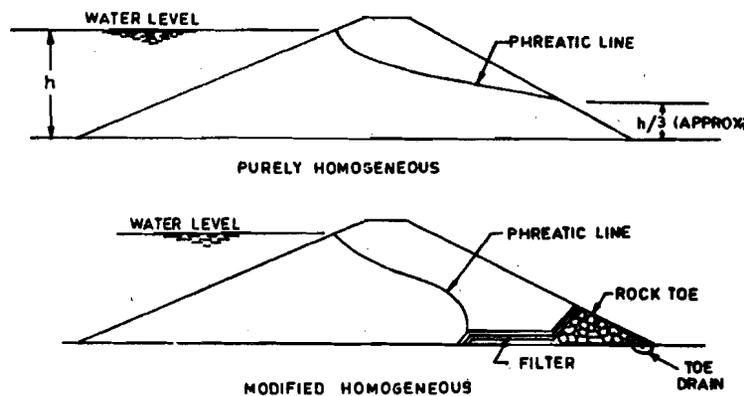
Figure 3.3 : Homogeneous Type Earth Dams
