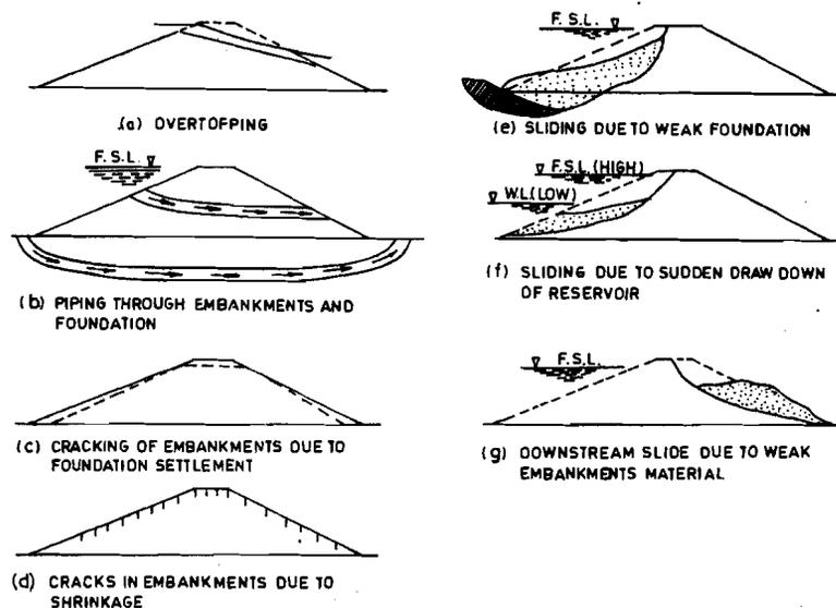
Figure 3.2 : Types of Failures – Earth Dams
