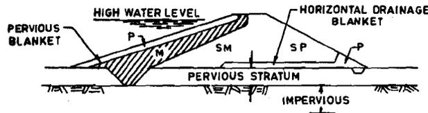
P = PERVIOUS, M = IMPERVIOUS, SM = SEMI-IMPERVIOUS, SP = SEMI-PERVIOUS
