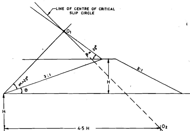
Figure 3.8 : Fellenius Method of Locating Line of Centre for Critical Slip Circle
