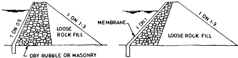
Figure 3.5 : Sections of Typical Rockfill Dams
