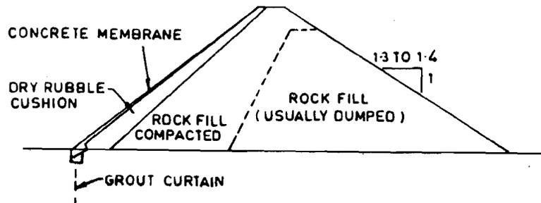
Figure 3.9 : Membrane Type Rockfill Dam
