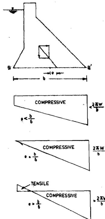
Figure 2.3 : Normal Stresses on the Base of a Gravity Dam
