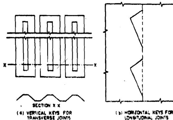
Figure 2.7 : Typical Keys for Joints in Gravity Dam
