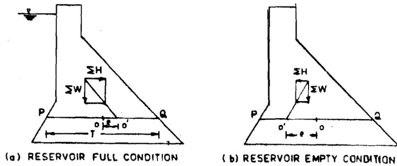
Figure 2.2 : Resultant Force on a Gravity Dam
