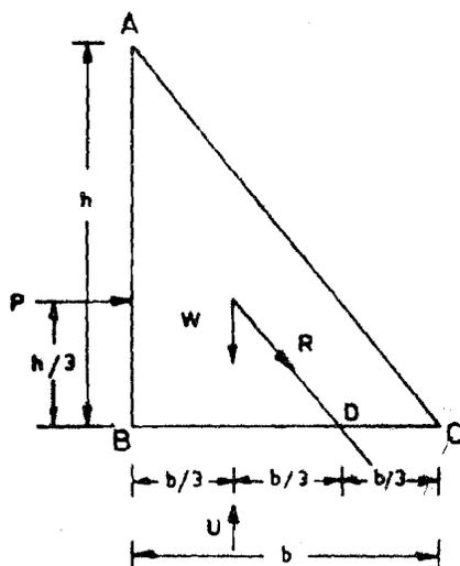
Figure 2.1 : Elementary Profile of a Gravity Dam
