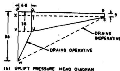
Figure 2.5 : Profile and Uplift Pressure Diagram for the Gravity Dam (Example 2.1)
