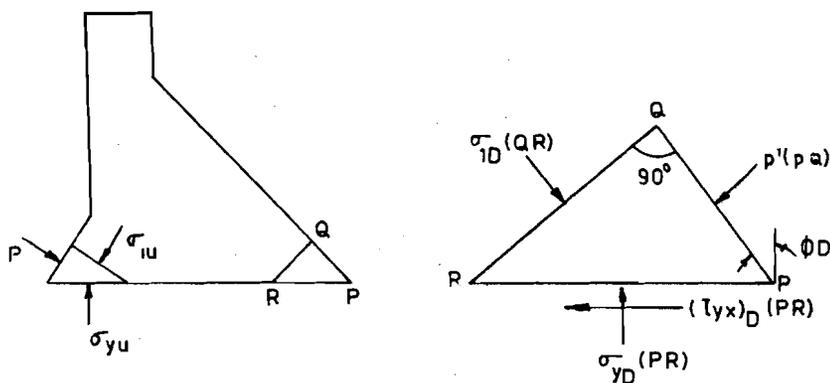
Figure 2.4 : Principal Stresses in a Gravity Dam
