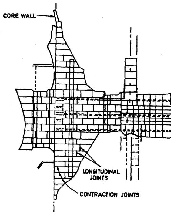
Figure 2.6 : Transverse and Longitudinal Joints in Bhakra Dam
