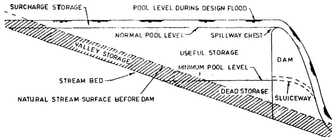
Figure 1.2 : Zones of Storage in a Reservoir
