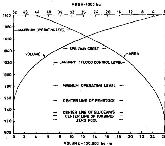
Figure 1.5 : A Typical Area-Capacity Curve of a Reservoir
