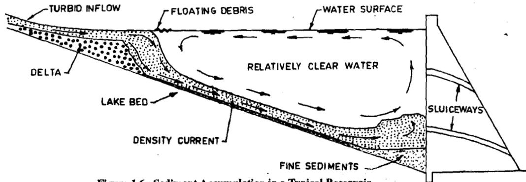
Figure 1.6 : Sediment Accumulation in a Typical Reservoir
