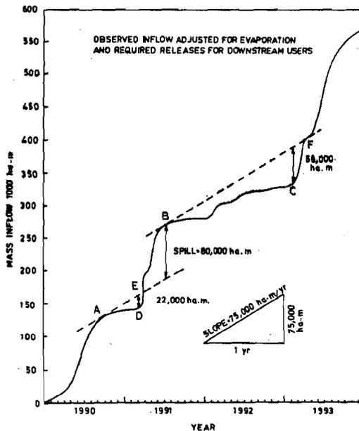
Figure 1.3 : Use of Mass Curve to Determine the Reservoir Capacity Required to Produce a Specified Yield (Example 1.1)
