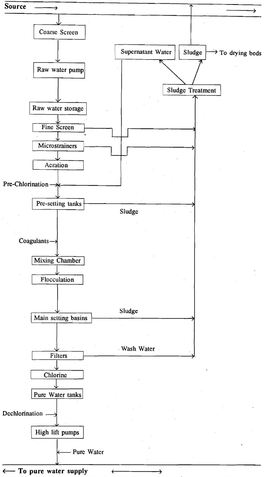
Figure 10.4 : Flow Diagram Showing Different Treatment Stages
