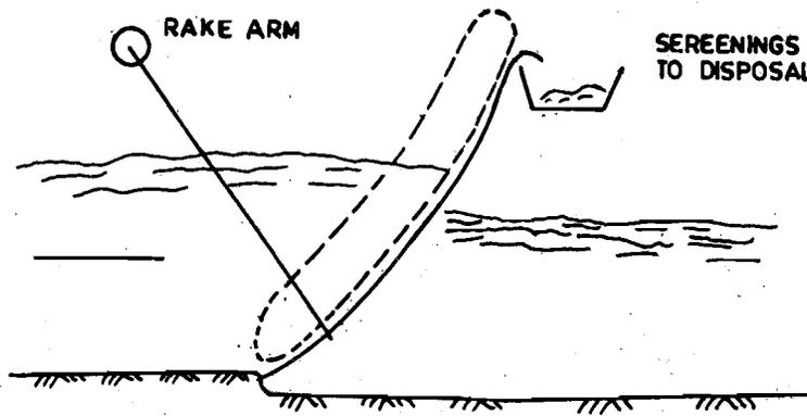
Figure 10.6 : Mechanically Racked Semi-rotary Screen
