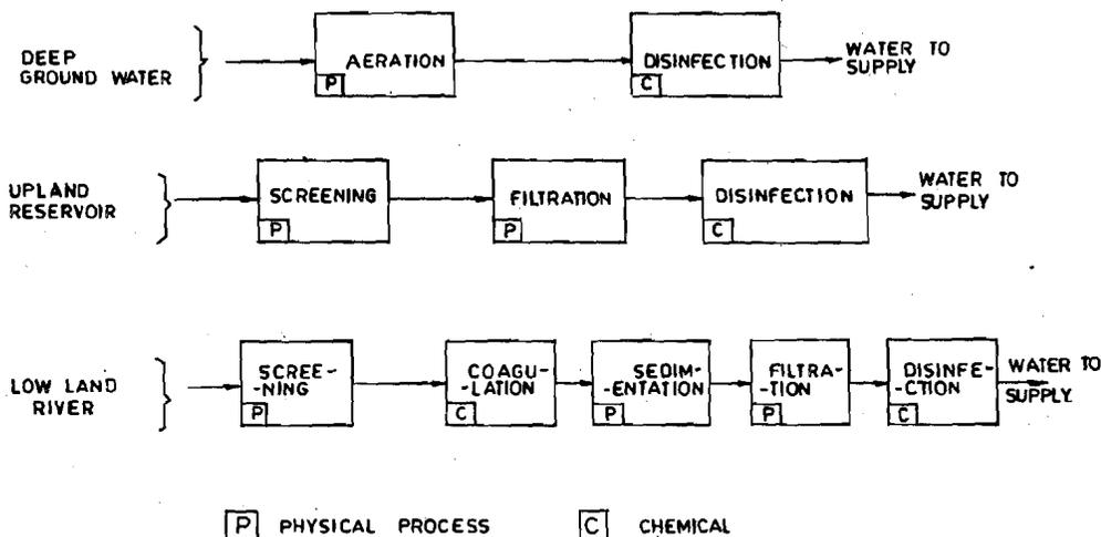
Figure 10.2 : Typical Water Treatment Processes
