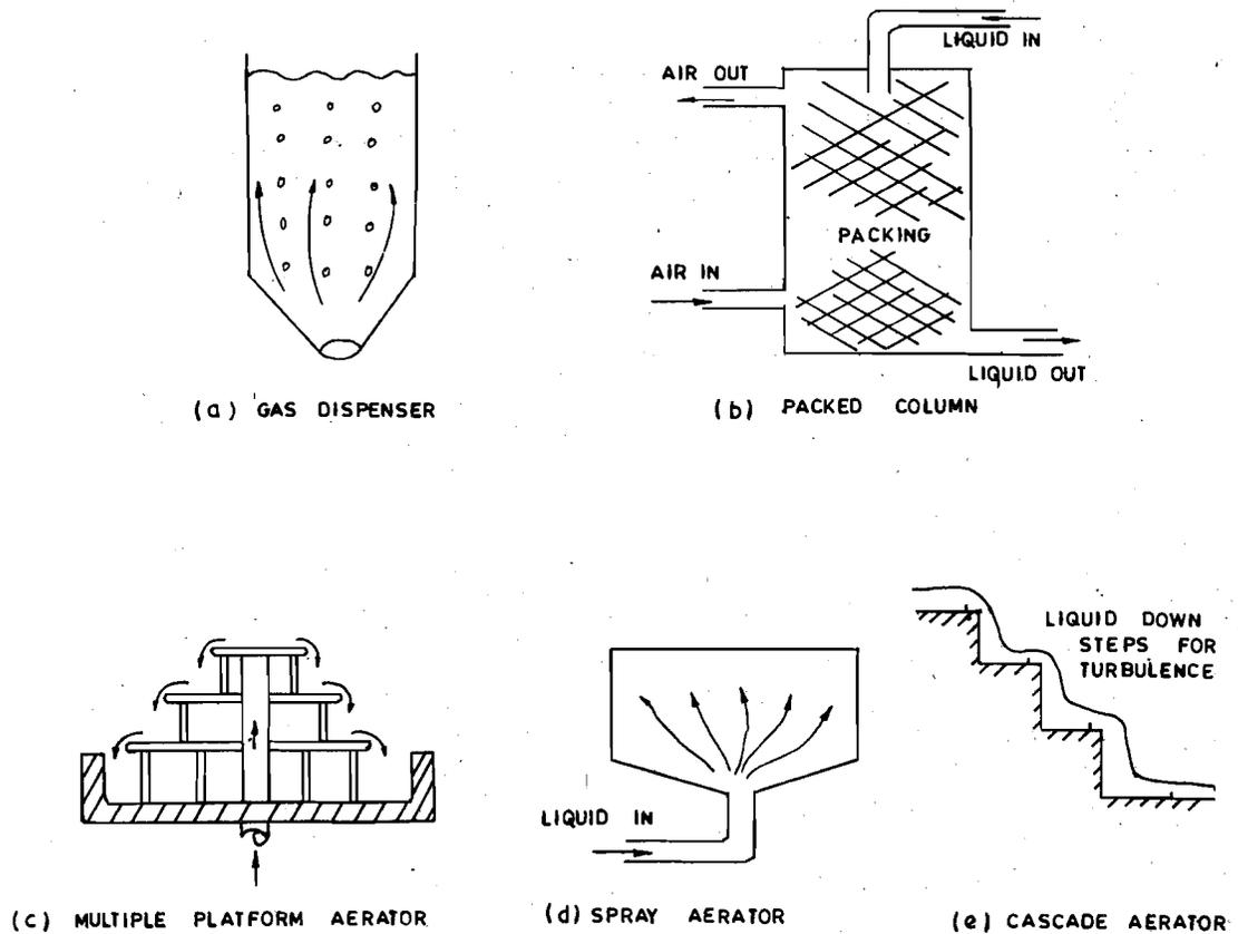
Figure 10.8 : Water Treatment Aeration Devices
