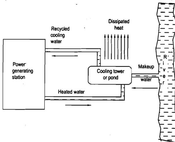
Figure 4.2 : Recirculation of Water to Control Thermal Pollution
