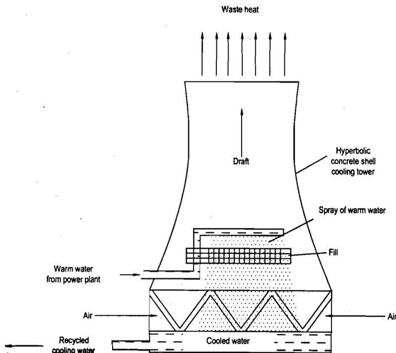
Figure 4.3 : A Schematic Sketch of Natural Draft Cooling Tower
