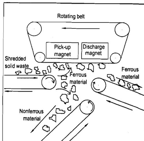
Figure 3.8 : Schematic Representation of a Magnetic Separator
