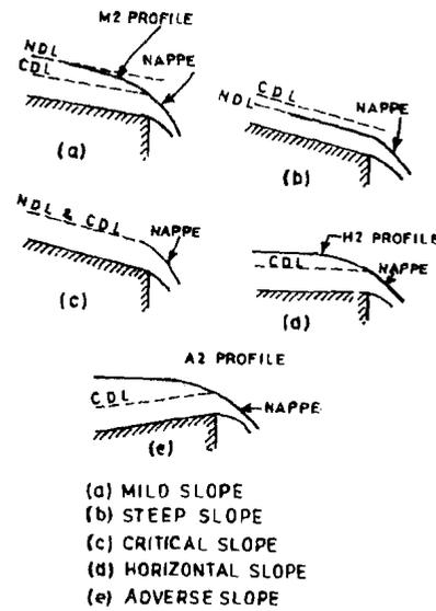
Figure 6.13 : Flow Profiles at Drops
