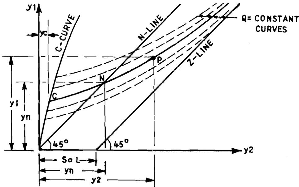
Figure 6.10 : Delivery of a Canal ( $Q$  - Constant Curves)
