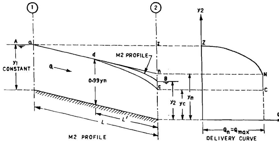
Figure 6.7 : Delivery of a Canal (Length of Canal more than Length of M2 Profile)
