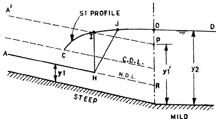
Figure 6.17 : Location of a Hydraulic Jump at a Junction of Steep and Mild Channels
