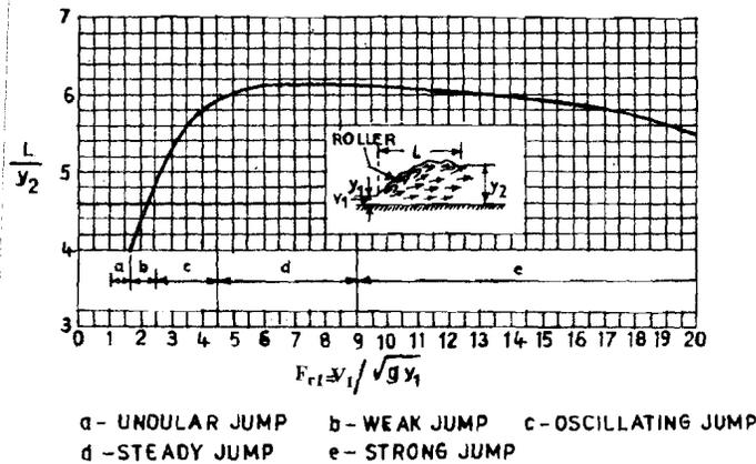
Figure 6.16 : Length, in terms of Sequent Depth of Jumps, in Horizontal Channels (Based on Data and Recommendations of U.S.B.R.)
