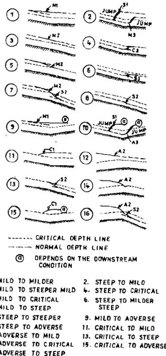
Figure 6.14 : Profiles in Channels with Break in Bed Slope
