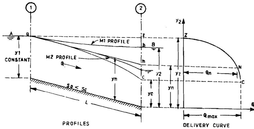
Figure 6.6 : Delivery of a Canal (Subcritical Flow with Upstream Depth Constant)
