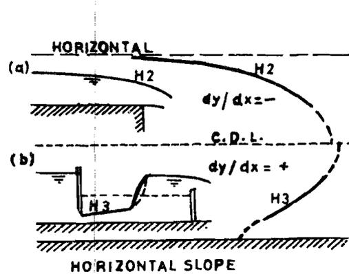
Figure 6.4 : Profiles in Horizontal Channels
