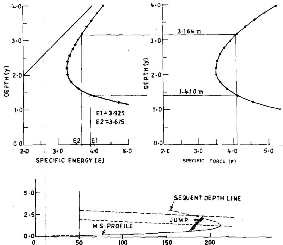
Figure 6.19 : Flow Profile for Example 6.2
