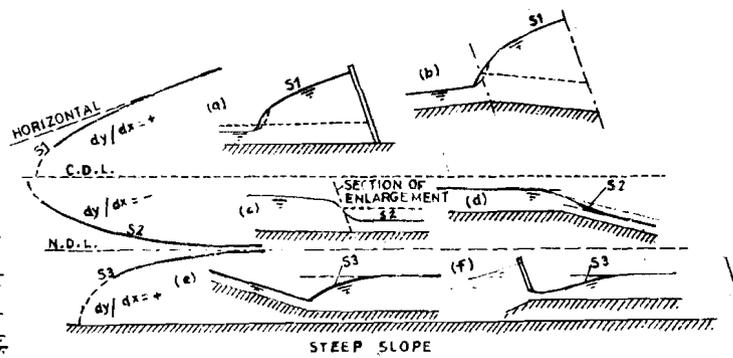
Figure 6.2 : Profiles in Steep Channels
