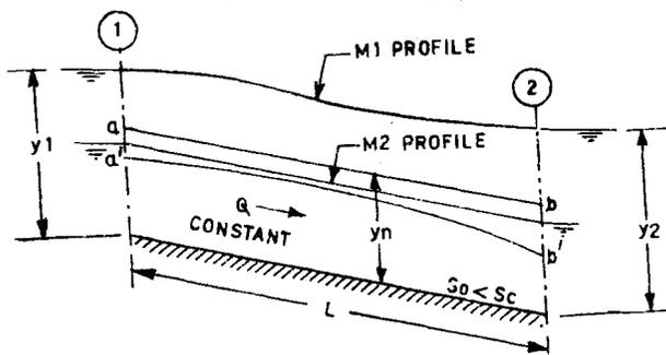
Figure 6.9 : Delivery of a Canal (Subcritical Flow with Constant Discharge)
