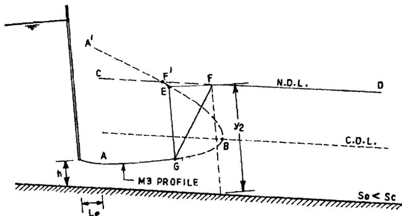
Figure 6.15 : Location of a Hydraulic Jump in a Mild Channel
