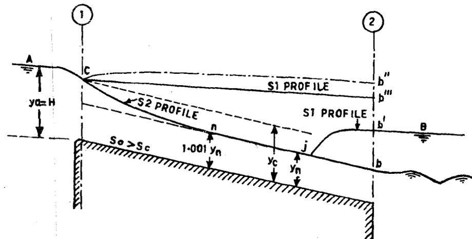
Figure 6.11 : Delivery of a Canal (Supercritical Flow)
