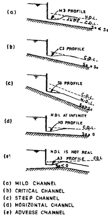
Figure 6.12 : Flow below a Sluice
