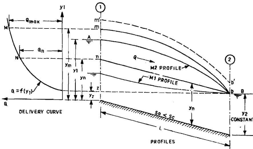
Figure 6.8 : Delivery of a Canal (Subcritical Flow with Downstream Depth Constant)
