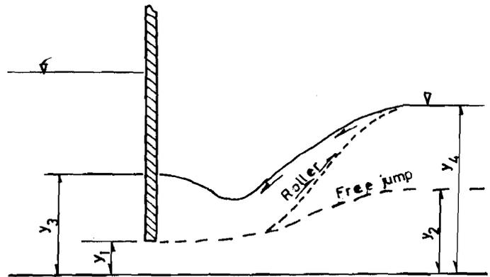
Figure 4.5 : A Submerged Hydraulic Jump at Sluice Outlet
