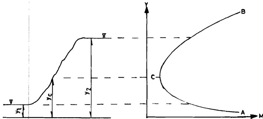
Figure 4.1 : Specific Momentum Curve and Sequent Depths  $y_1$  and  $y_2$  of a Hydraulic Jump
