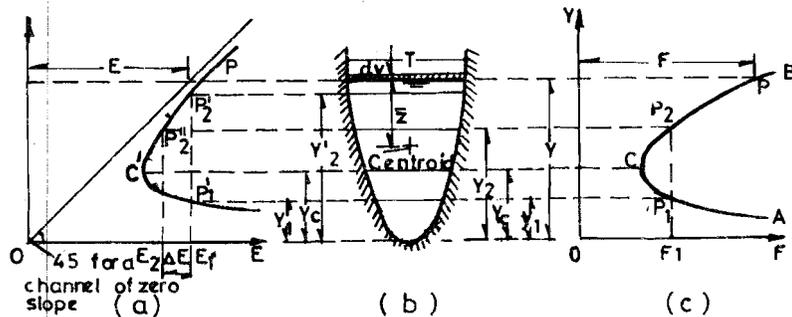
Figure 4.2 : Specific Force Curve in Comparison with Specific Energy Curve
