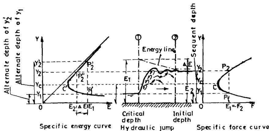
Figure 4.3 : Hydraulic Jump Interpreted by Specific Energy and Specific Force Curves
