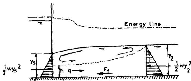
Figure 4.4 : Definition Sketch of a Submerged Hydraulic Jump
