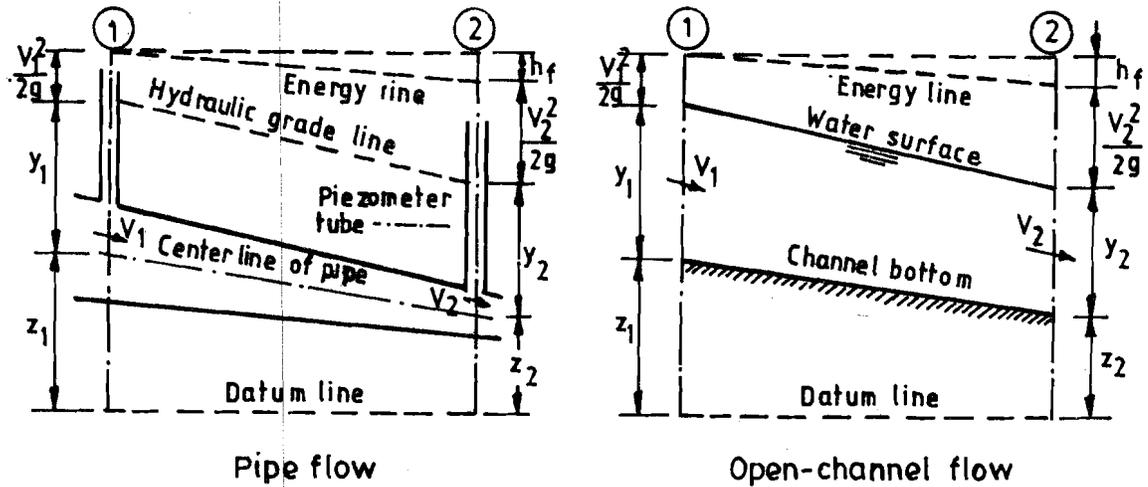
Figure 1.1 : Comparison Between Pipe Flow and Open Channel Flow
