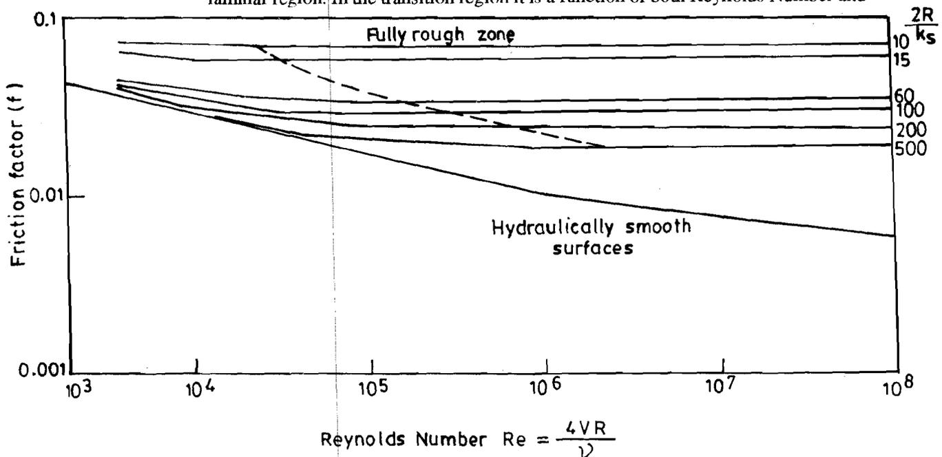
Figure 1.3 : Modified Moody Diagram Showing the Behaviour of the Friction Factor in Open Channel Flow
