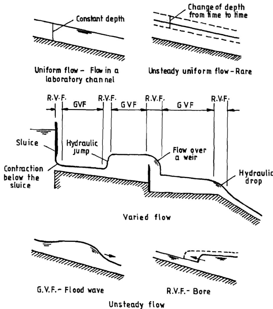
Figure 1.2 : Various Types of Open Channel Flow
