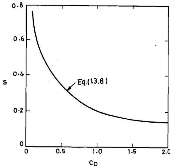
Figure 13.9 : Variation of  $S$  with  $C_D$  for a Cylinder
