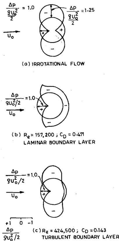
Figure 13.5 : Pressure Distribution around a Sphere
