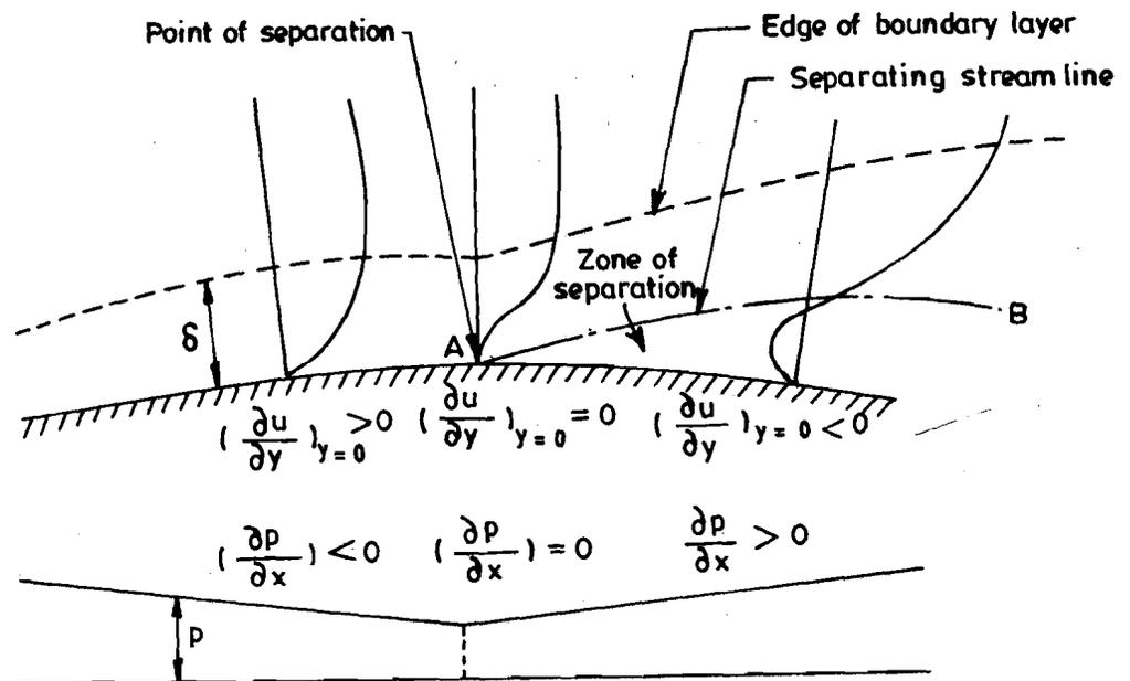
Figure 13.1 : Separation of Boundary Layer in an Expanding Flow
