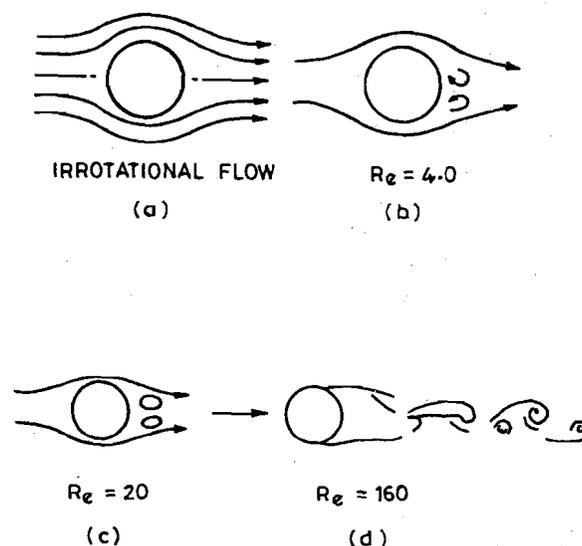
Figure 13.7 : Flow around an Infinite Cylinder
