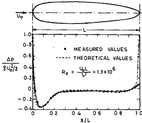
Figure 13.12 : Pressure Distribution around an Airfoil
