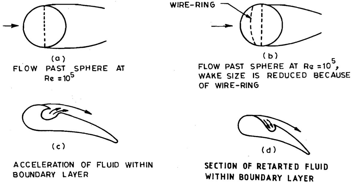
Figure 13.2 : Methods of Boundary Layer Control
