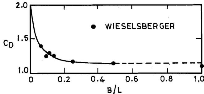
Figure 13.11 : Variation of  $C_D$  with  $B/L$  for a Rectangular Plate held Perpendicular to the Flow
