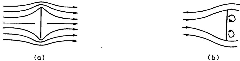
Figure 13.10 : Flow Pattern around a Flat Plate
