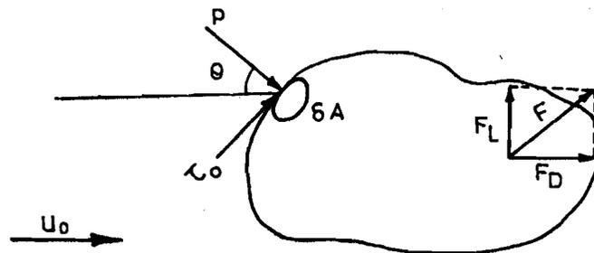
Figure 13.4 : Definition of Drag and Lift
