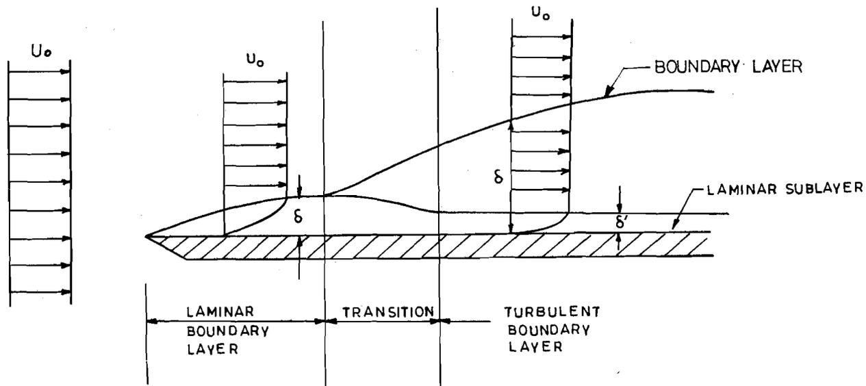
Figure 10.3 : Development of Boundary Layer over a Flat Plate
