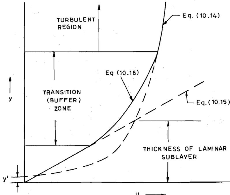
Figure 10.6 : Velocity Distribution in Different Zones
