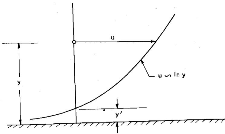
Figure 10.5 : Logarithmic Velocity Distribution in Turbulent Flow
