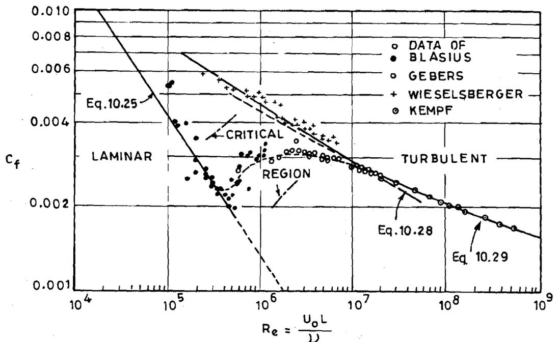
Figure 10.7 : The Mean Drag Coefficient for a Plane Boundary as a Function of the Reynolds Number
