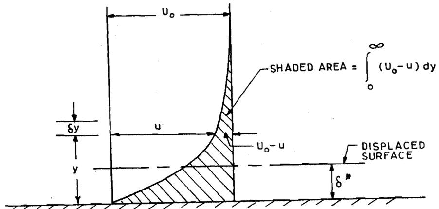
Figure 10.2: Displacement Thickness
