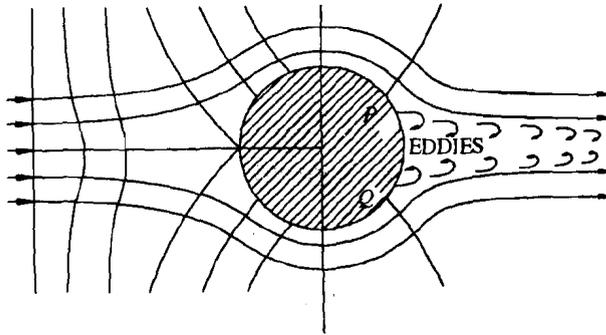
Figure 4.11 : Actual flow pattern for flow over a cylinder (Real fluid flow)
