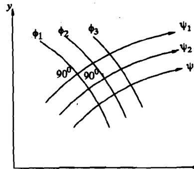
Figure 4.8 : Flow net for a 2-dimensional flow
