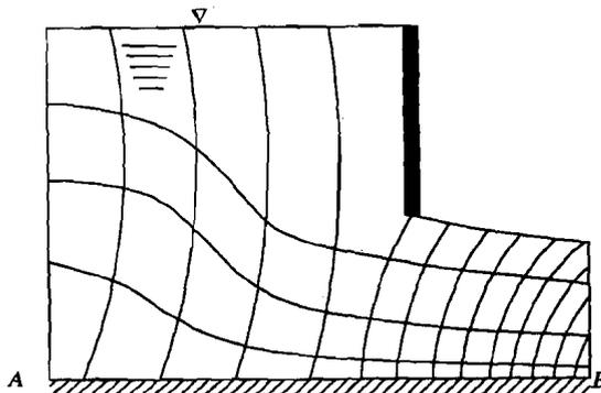
Figure 4.12 : Flow through sluice outlet
