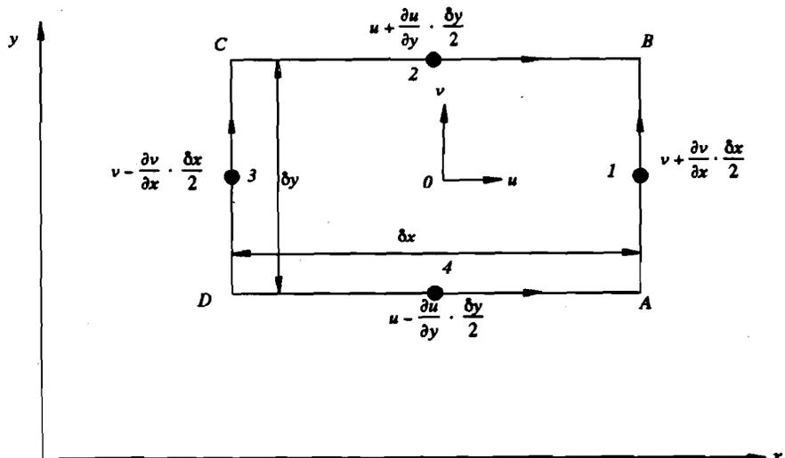
Figure 4.5 : Circulation in  $x - y$  plane
