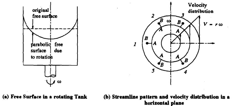
Figure 4.6 : Characteristics of a Forced-vortex
