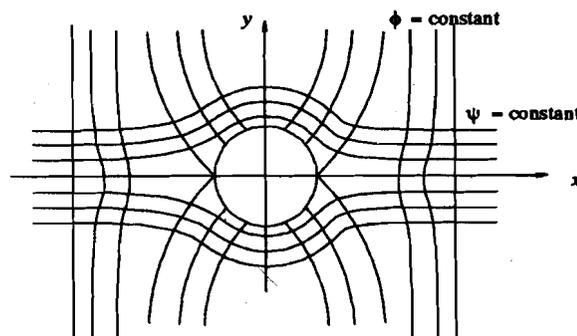
Figure 4.10 : Flow net for a flow past a cylinder (Irrotational flow)
