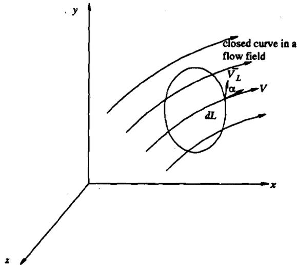
Figure 4.4 : Circulation around a curve
