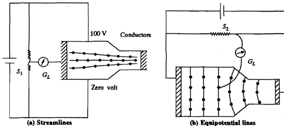
Figure 4.9 : Electrical analogy method
