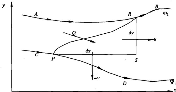
Figure 4.1 Relationship between velocity components and stream function
