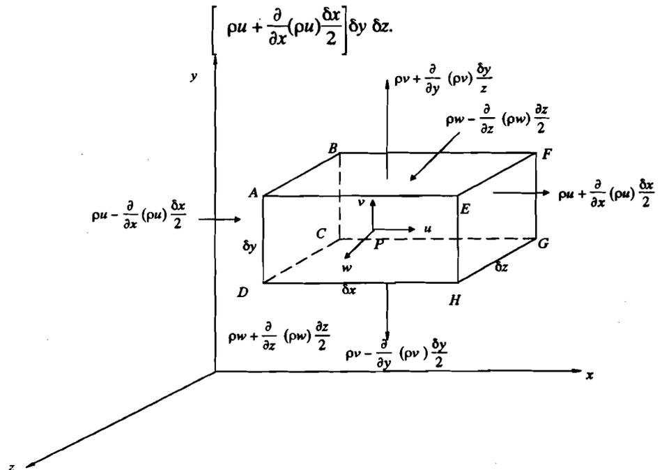
Figure 3.12 : Mass flow in and out of the rectangular parallelepiped
