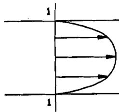
Figure : 3.5 (b) Velocity in laminar flow (Real fluid)
