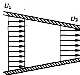
(a) Steady ideal fluid flow through a converging section
