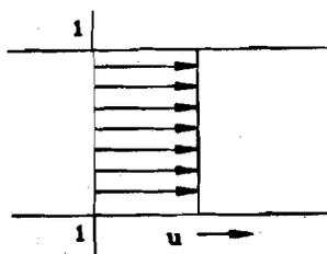
Figure 3.5 (a) Velocity in an ideal fluid (slip condition at the boundary)
