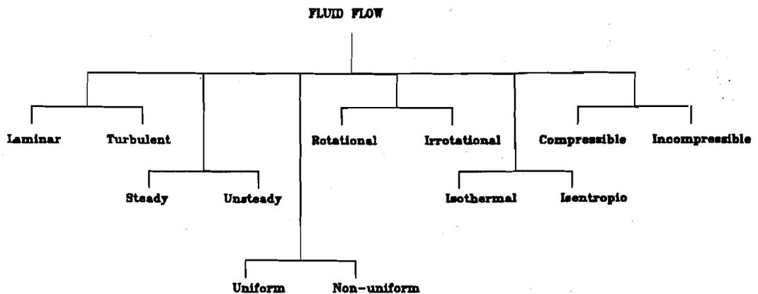
Figure 3.1 : Classification of Fluid Flow
