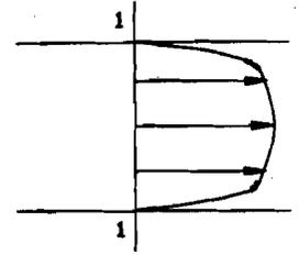
Figure 3.5 (c) Velocity in turbulent flow (Real Fluid)
