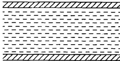
Figure 3.2 (a) : Laminar Flow
