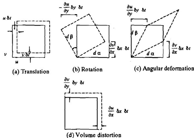
Figure 3.11 : Changes the fluid element undergoes while in motion
