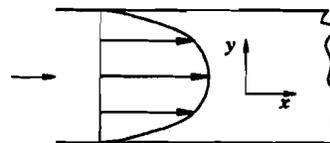
(b) Steady flow through a pipe
