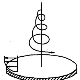
(c) Steady flow rotating in a fixed wall
