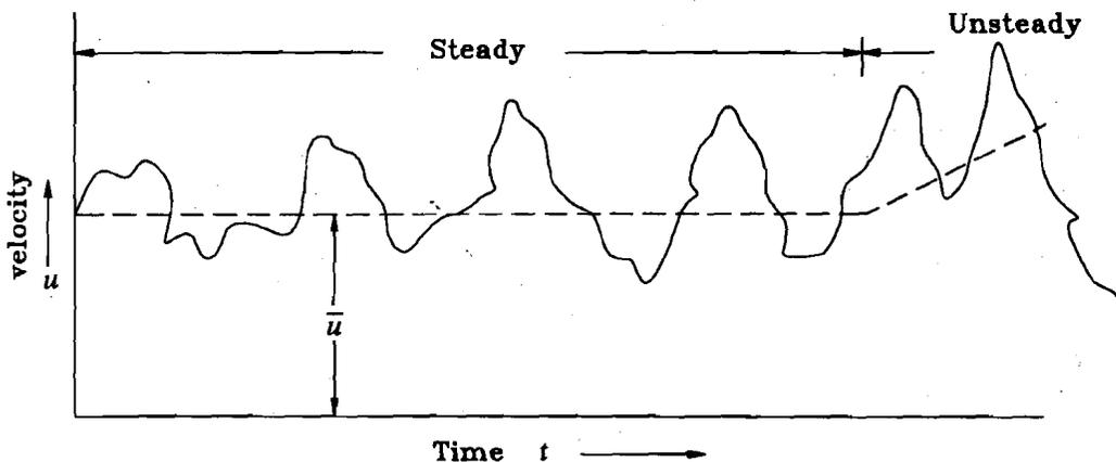
Figure 3.4: Turbulent flow - Temporal Mean Velocity
