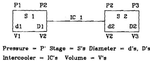
Figure 11.9 : Operating Principle of a Two-stage Compression
