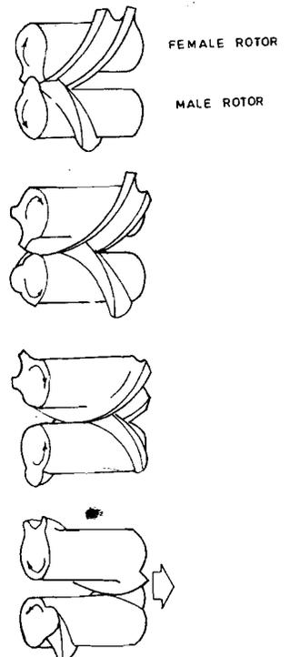
Figure 11.7 : Working Principle of a Screw Compressor (Simplified)
