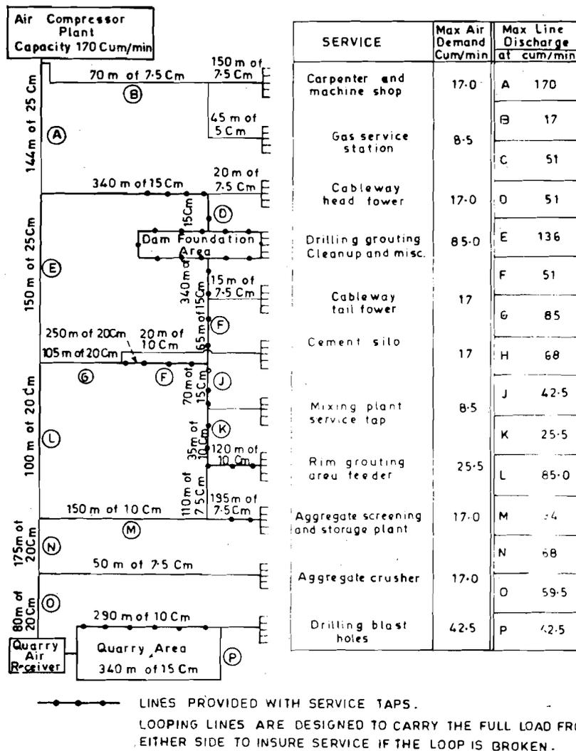
Figure 11.2 : Compressed Air Distribution System for Large Construction Job
