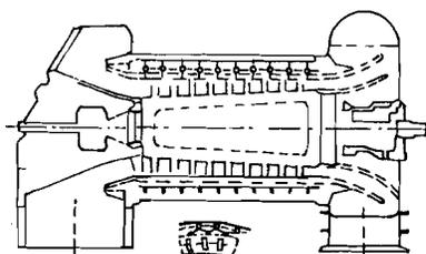
Figure 11.3 : Axial Compressor
