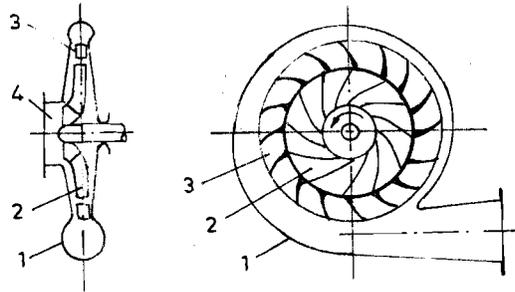
**Figure 11.12 : Centrifugal Single-stage Blower**
