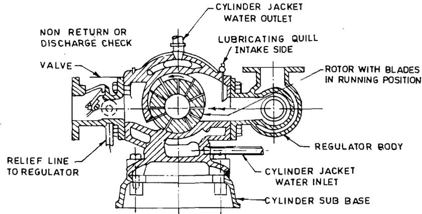
Figure 11.8 : Sectional End View of a Sliding Vane Rotary Compressor
