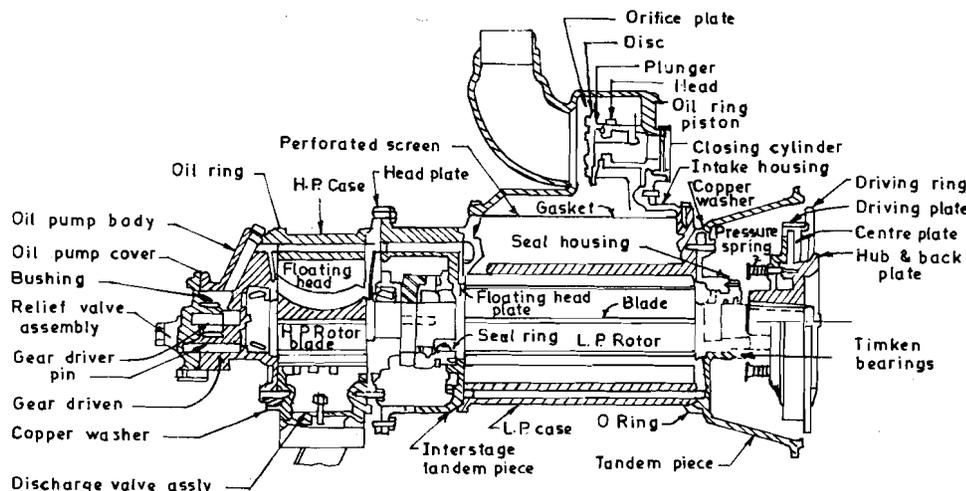
Figure 11.6 : Sectional View of Rotary Air Compressor
