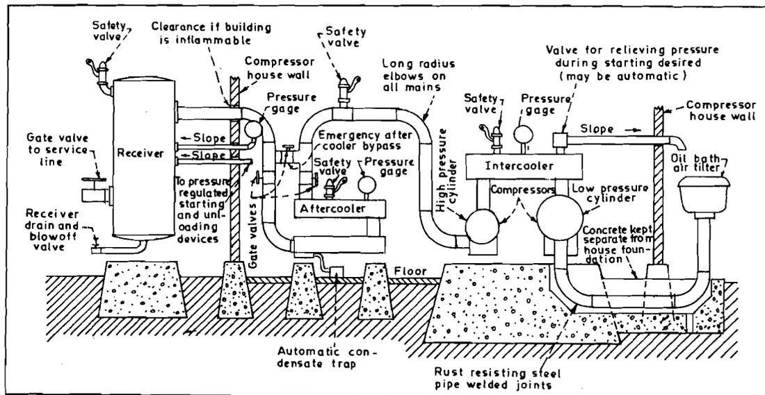
Figure 11.1 : Diagrammatic Layout of Stationary Air Compressor System
