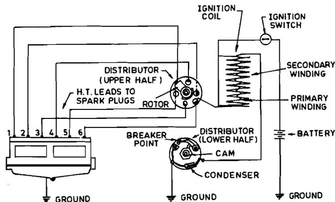
Figure 10.3 : Battery Type Ignition System for a Petrol Engine
