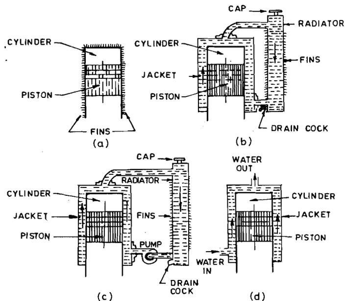
**Figure 10.6 : Methods of Engine Cooling**
