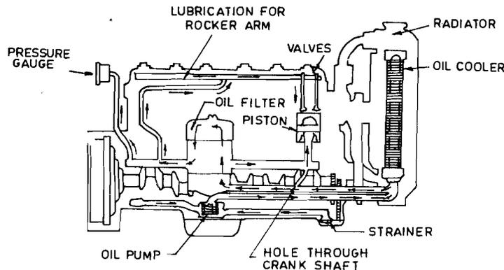
Figure 10.5 : Pressure Lubrication System of an IC Engine
