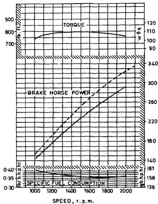
Figure 10.1 : Performance Curves for a Diesel Engine
