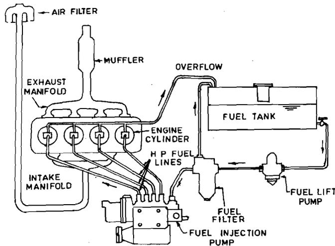
Figure 10.4 : Fuel System for a Diesel Engine
