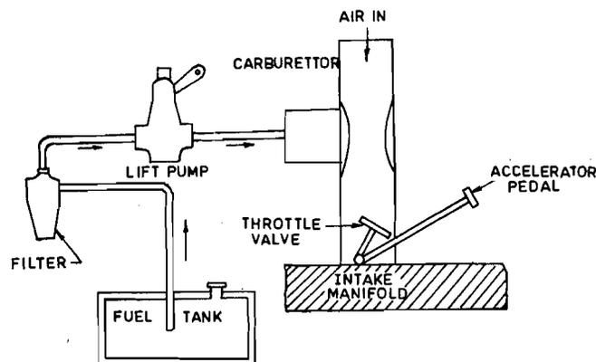
Figure 10.2 : Fuel System of a Spark Ignition Engine
