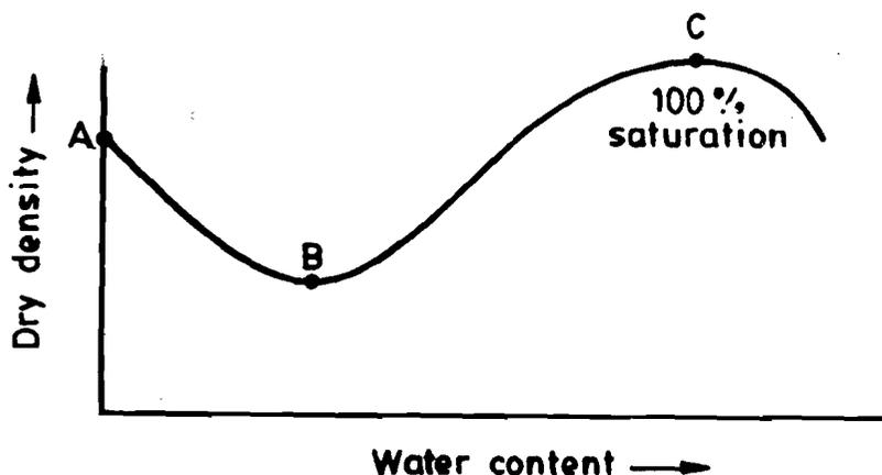
Figure 17.3 : Typical Moisture Density Curve for Cohesionless Soil
