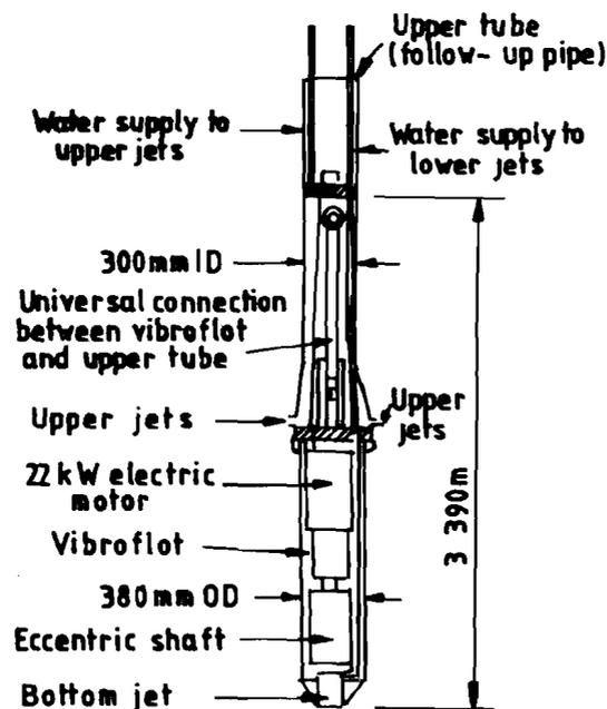
Figure 17.8 : Diagram of Vibroflot
