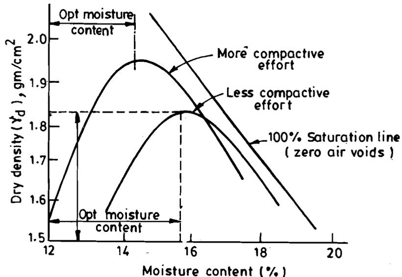
Figure 17.1 : Moisture Density Curve
