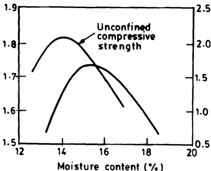
Figure 17.2: Moisture-density and Shear Strength Moisture Curve – a Comparison
