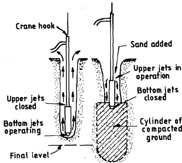
(a) Jetting down Vibroflot (b) Withdrawal of Vibroflot
