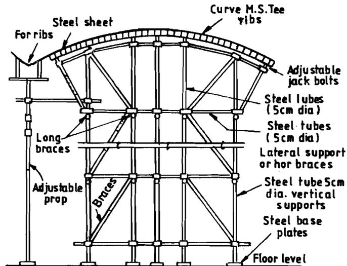
Figure 16.8 : Tubular Steel Formwork for Barrel Shell-roofs
