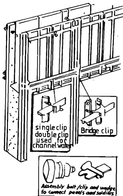
Figure 16.6 : Wallform Climbing Steel Shuttering
