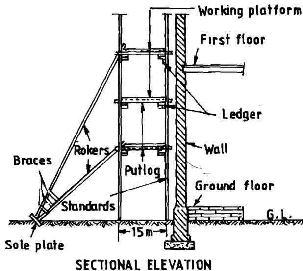
Figure 16.16 : Details of Double or Mason's Scaffolding with Raking Shore
