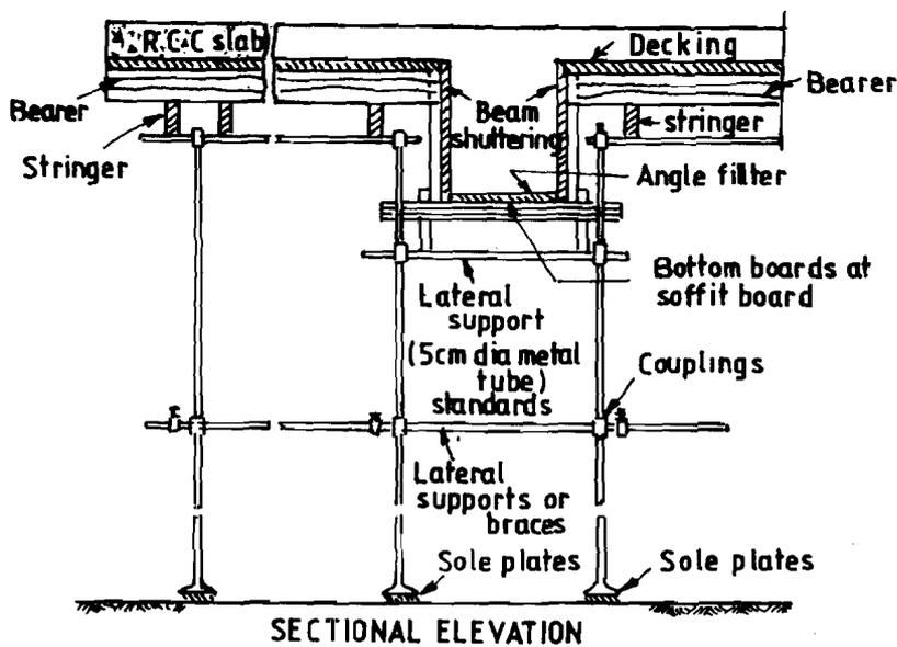
Figure 16.17 : Details of Tabular Steel Scaffolding Used as Centering for Slab and Beam Construction
