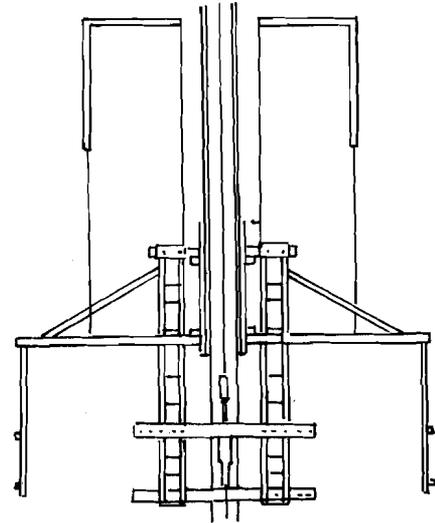
Form panels, straight or curved, are fitted to sturdy yokes with working platform, suspended walkways and safety railings Hydraulic jacks mounted on yoke beams climb on solid jack rods. The slipform is available for tapered structures also.
