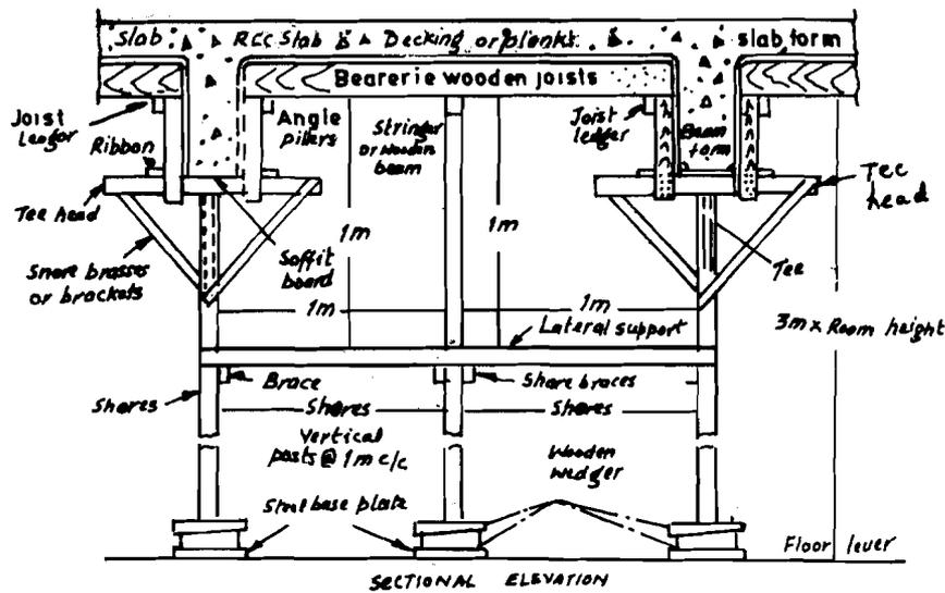
Figure 16.2 : Wooden Formwork for Monolithic R.C.C. Beam and Slab Floor
