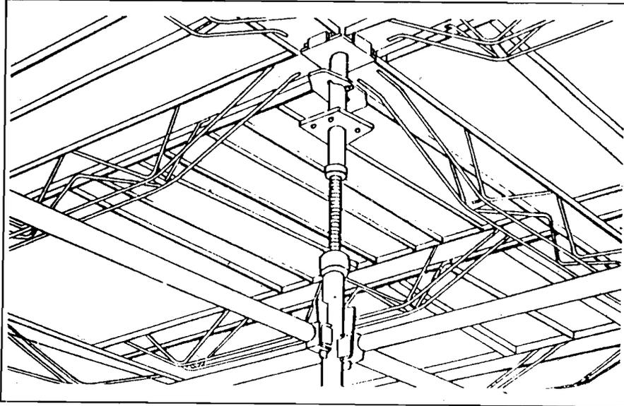
Figure 16.5 : Grid Decking System
