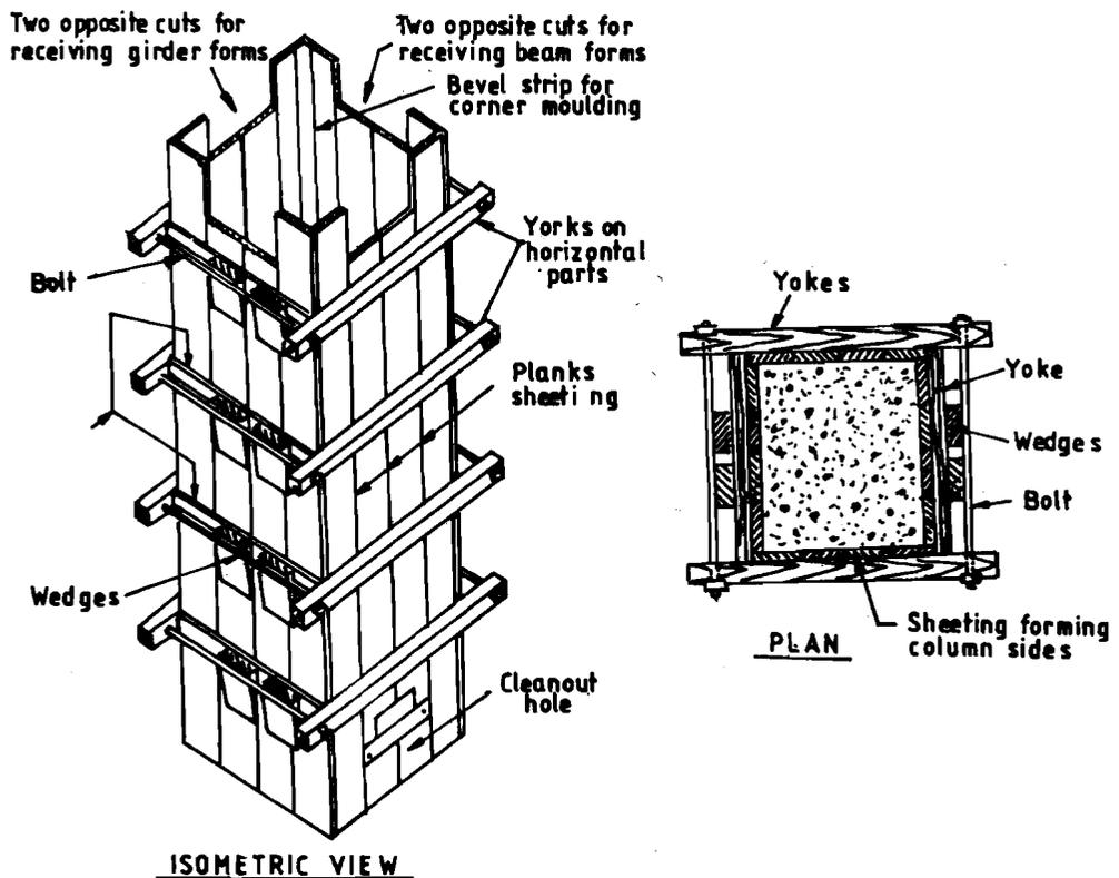
**Figure 16.1 : Formwork for Column**
