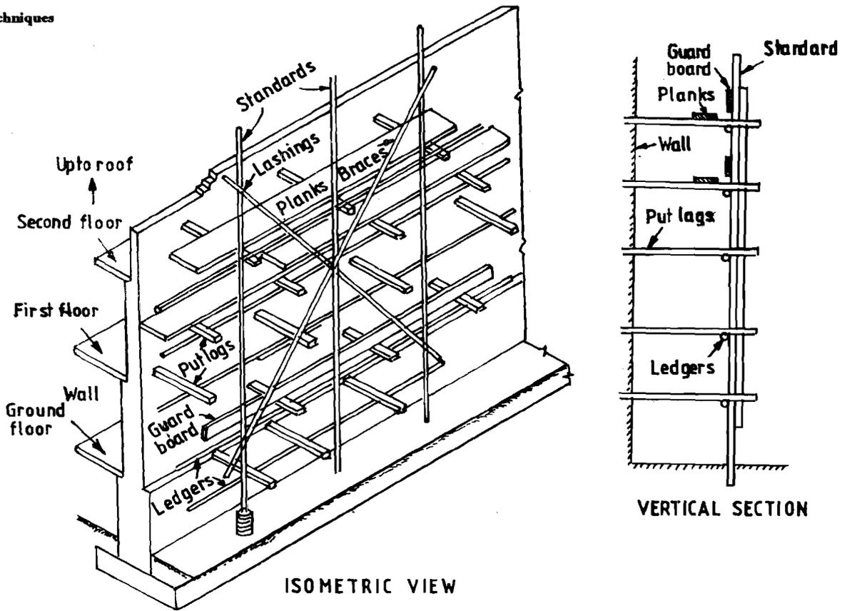
Figure 16.15 : Scaffolding and its Various Parts
