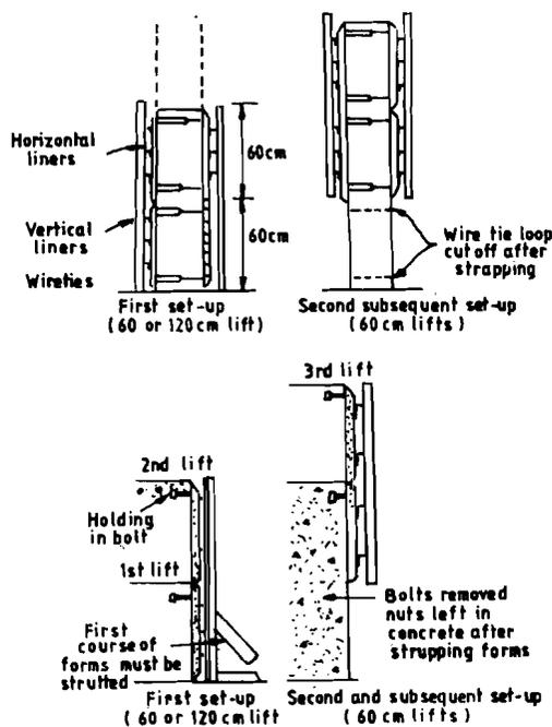
Figure 16.10 : Climbing Formwork of Steel Forms for Thick Walls
