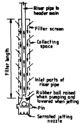
Figure 14.2 : Diagrammatic Arrangement of a Wellpoint
