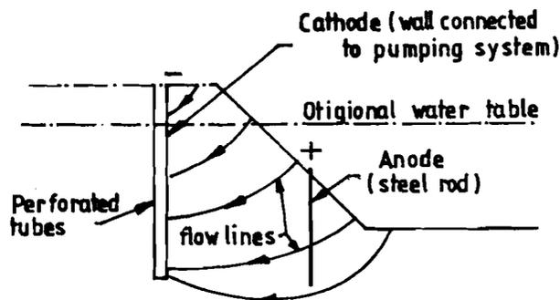
Figure 14.7 : Electro-Osmosis Installation
