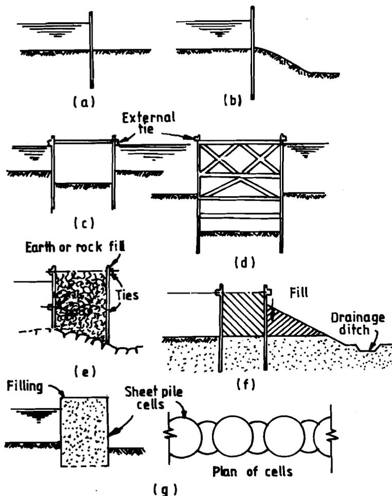
(a) Single Wall (b) Single Wall with Earth Bank (c) With Single Top Frame
