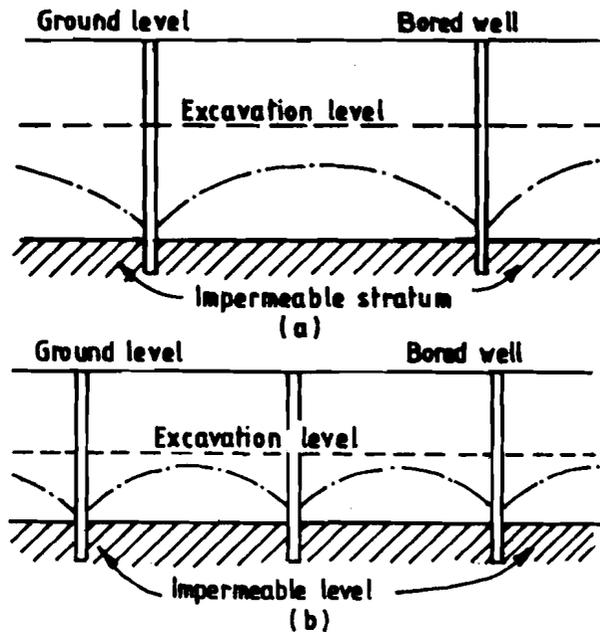
Figure 14.6 : Spacing of Bored Wells
