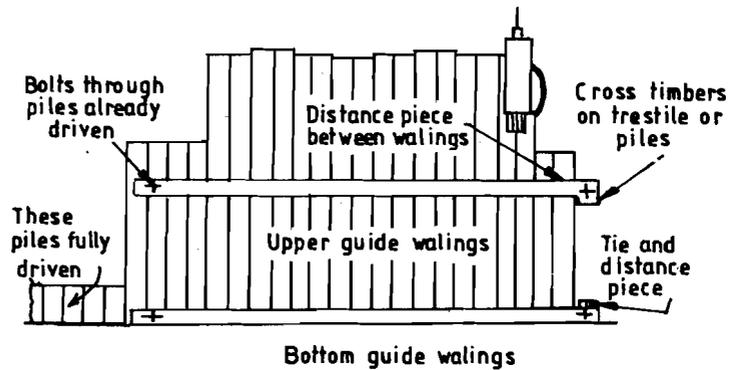
Figure 14.10 : Guide Wallings for Driving Sheet Piles
