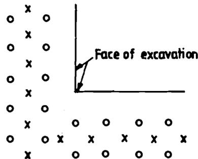
Figure 14.8 : Layout Plan of Grout Injection Holes to Form 'Grout Curtain' Around Excavation. o, Primary Injection Holes; x, Secondary Injection Holes.
