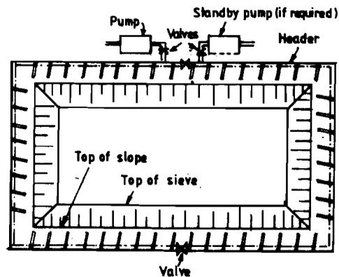
Figure 14.4 : Single-stage Wellpoint Installation by the Ring System
