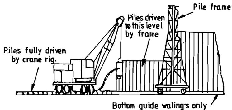
Figure 14.11 : Typical Two-stage Pile Driving
