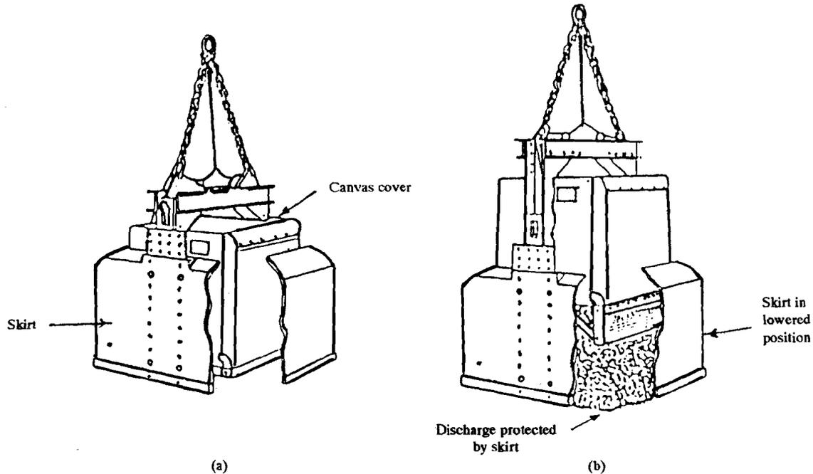
Figure 12.4 : Placement with the Bottom Dump Bucket : (a) Filled; (b) Discharging.
