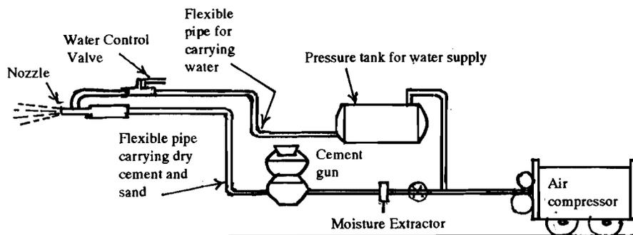
Figure 12.9 : A Typical Plant Layout of Guniting Equipment
