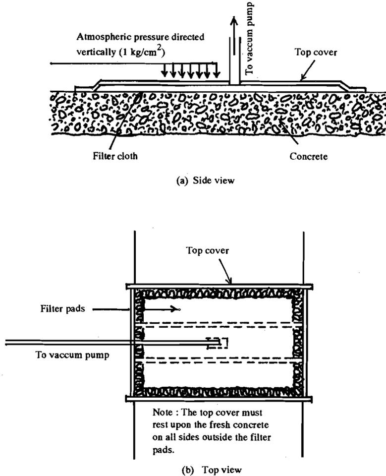
Figure 12.6 : Vacuum Dewatering
