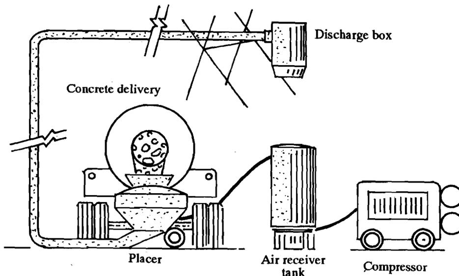
Figure 12.2 : Pneumatic Pump
