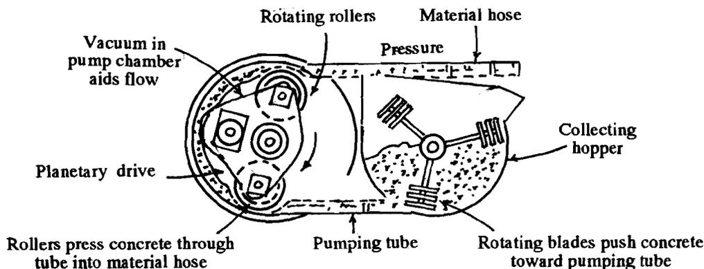
Figure 12.3 : Squeeze Pressure Pump
