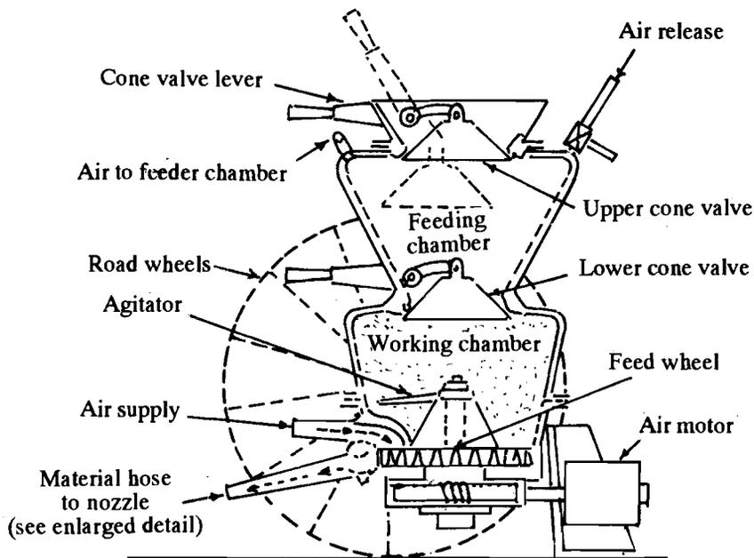
Figure 12.8 : Schematic View of Shotcreting Equipment
