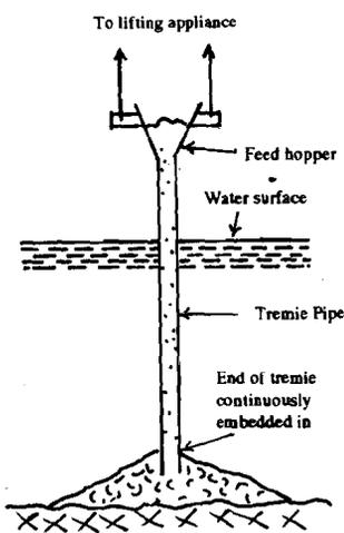
Figure 12.5 : Tremie Method of Concreting
