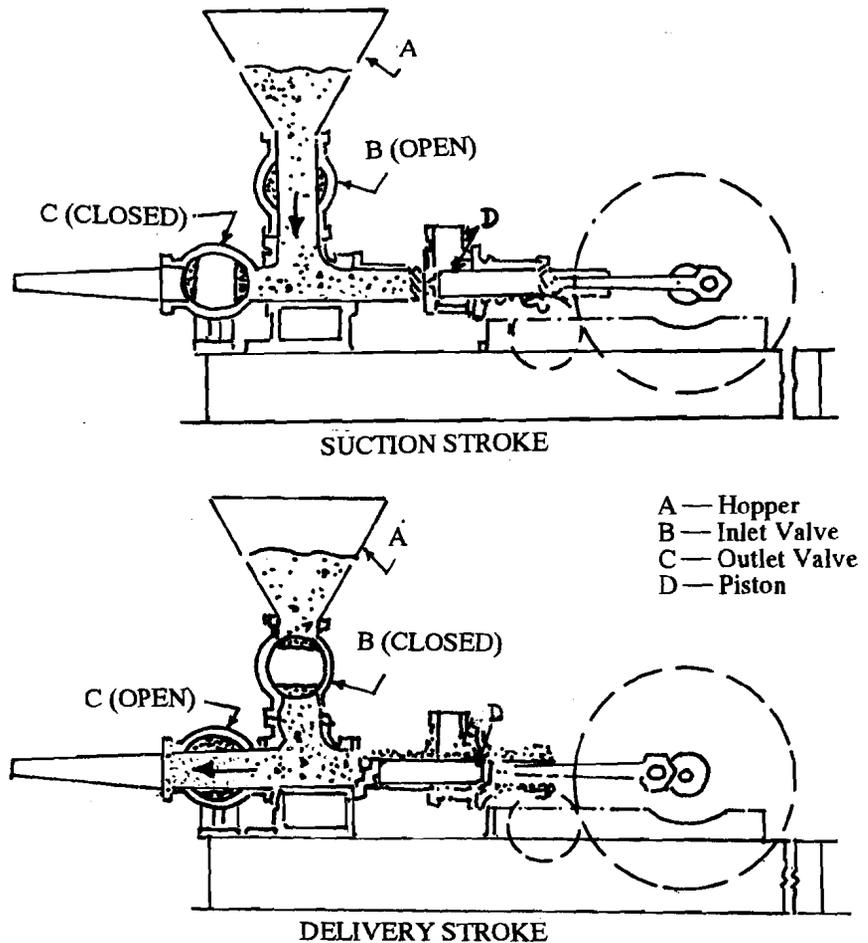
Figure 12.1 :The Working Cycle of the Piston Concrete Pump
