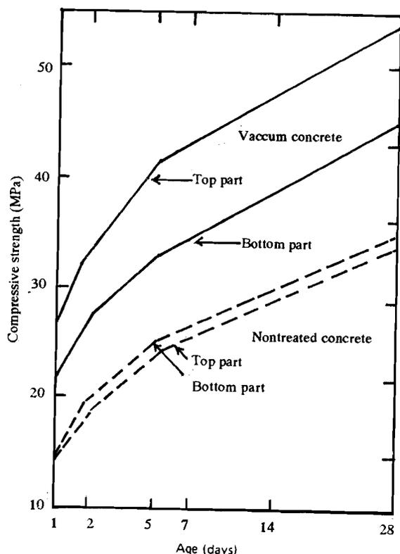
Figure 12.7 : Effect of Vacuum Dewatering on the Strength of Concrete
