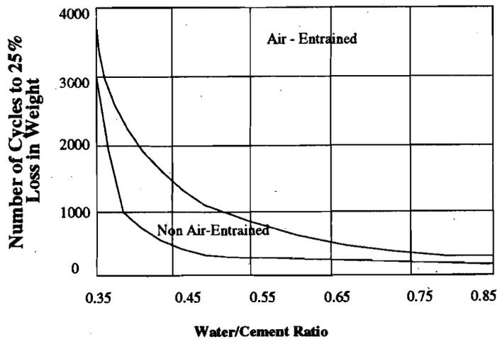
Fig. 8.1 : Influence of Water/cement Ratio on The Frost Resistance of Concrete Moist-cured For 28 Days.
