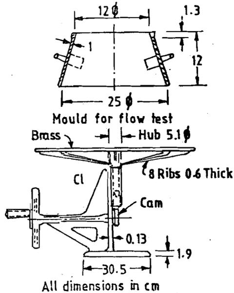
Figure 5.4 : Flow Test Apparatus
