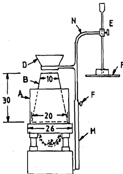
Figure 5.6 : Vee-Bee Consistometer
