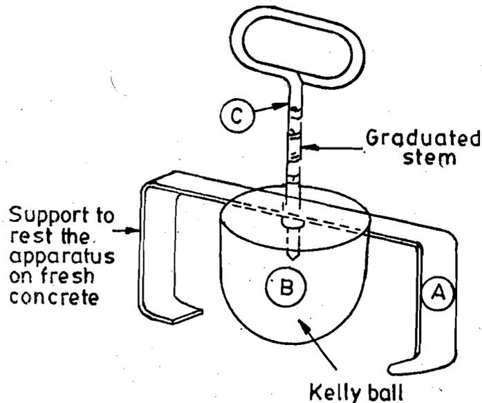
Figure 5.5 : Kelly Ball Test Apparatus
