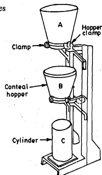
**Figure 5.3 : Compacting Factor Test Apparatus**
