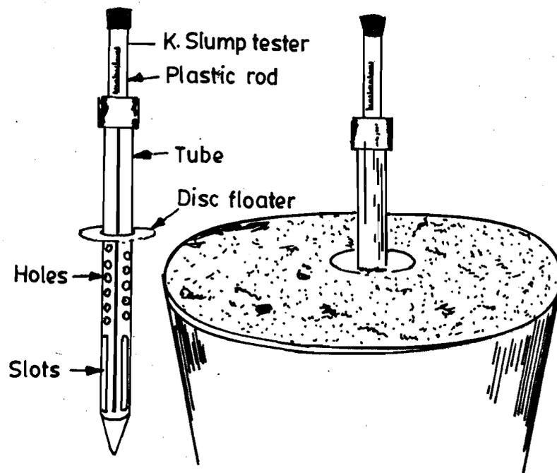
Figure 5.2 : K - Slump Test Apparatus
