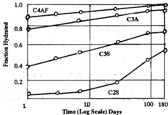
Figure 1.1: Rate of Hydration of the Cement Compounds
