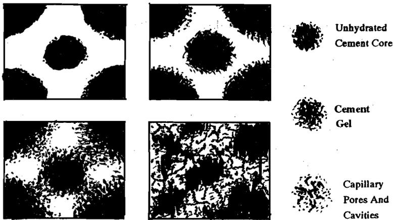
Figure 1.2 : Diagrammatic Representation of the Hydration Process and Formation of Cement gel
