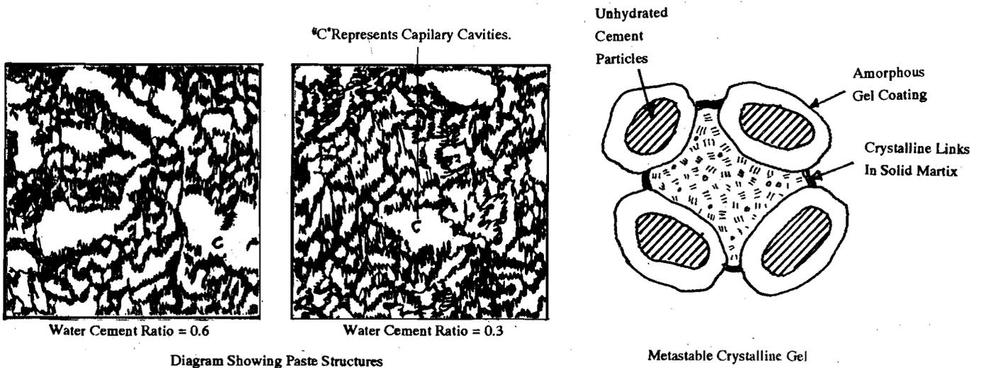
Figure 1.3 : Microscopic Schematic Model Representing the Structure of Hardened Cement Paste
