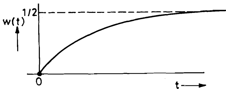
Fig. 5.9 : Step-response w(t) of the system with H(s) = \frac{1}{s + 2}
