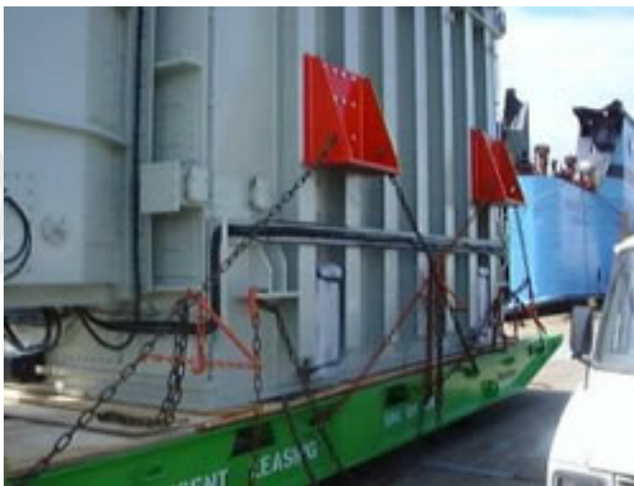
Figure 3.14 : Picture Showing Securing of a Heavy Cargo with Lashing Chain
