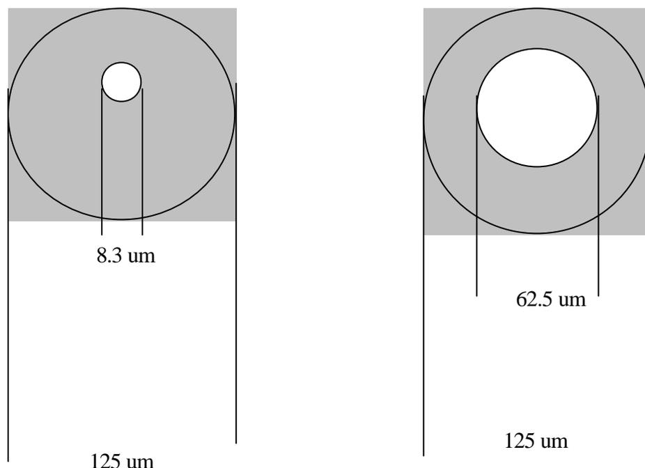
Figure 7: Single Mode Fibre
