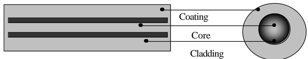
**Coating:** The outer layer of the fibre is coating. Generally made of an acrylate material, the coating has no affect on the transmission properties. It protects the fibre when it is being processed into a cable and when being handled during installation and termination
