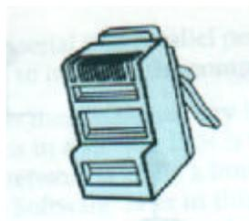
Figure 5: RJ - 45 Connector
