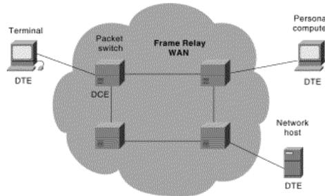
**Figure 5 : DCEs Generally Reside Within Carrier-Operated WANs**
