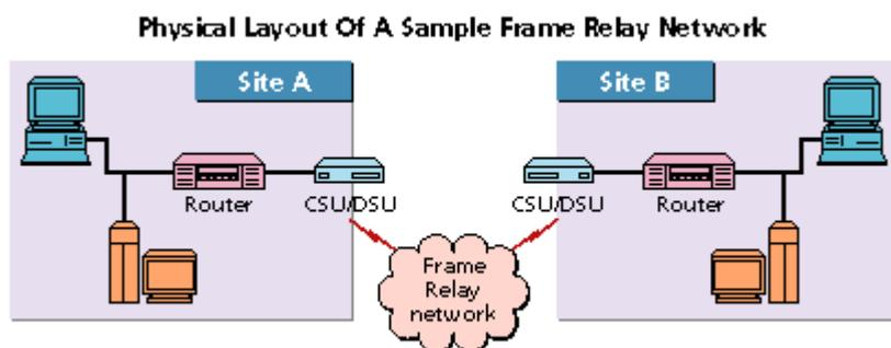
Figure 4: Frame Relay Network
