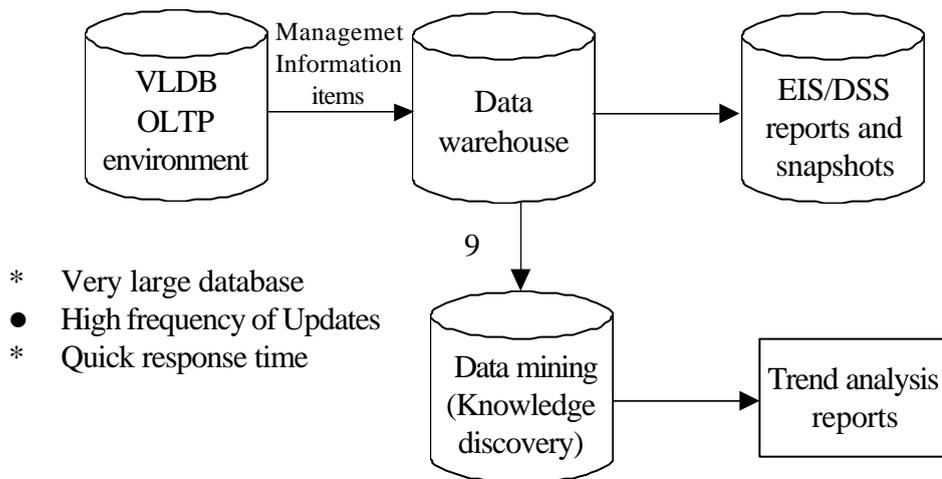
**Fig. 4.7 : A schematic of data warehousing and data mining**
