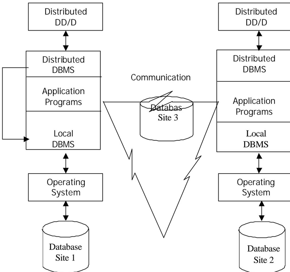
**Fig: 4.1 : Architecture and schematic representation of a distributed database**
