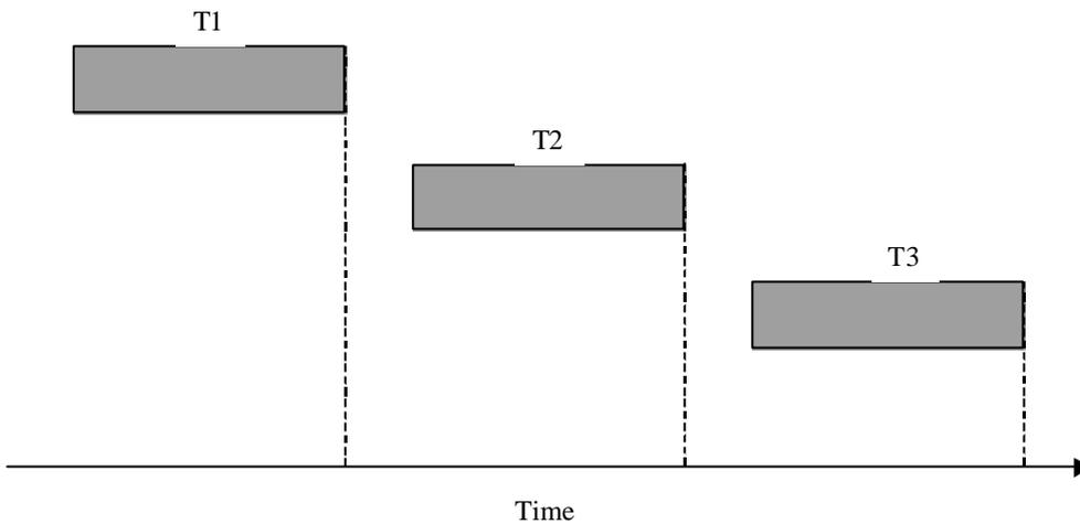
**Fig. 4.4 : Serial execution of transactions**
