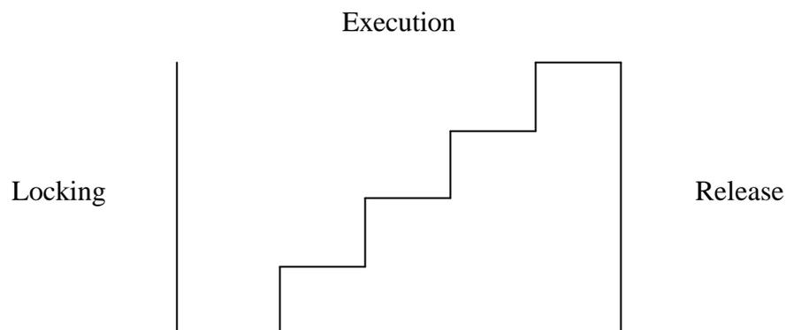
Fig. 4.6 : Three phases of a transaction. Incremental locking and simultaneous release
