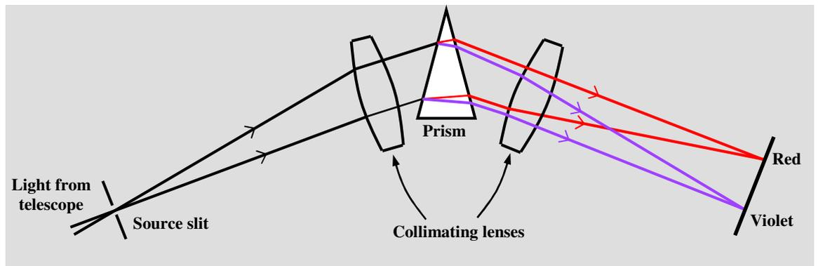
Fig.7.8: Schematic diagram of a spectroscope
