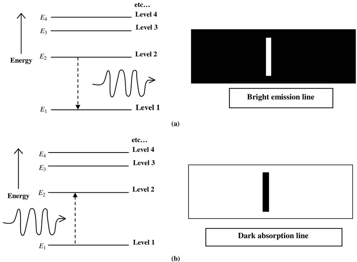
**Fig.7.3: The atomic electron a) emits radiation when it makes a transition from a higher energy level to a lower energy level giving rise to emission spectrum; and b) makes a transition to a higher energy level on absorbing radiation giving rise to absorption spectrum**
