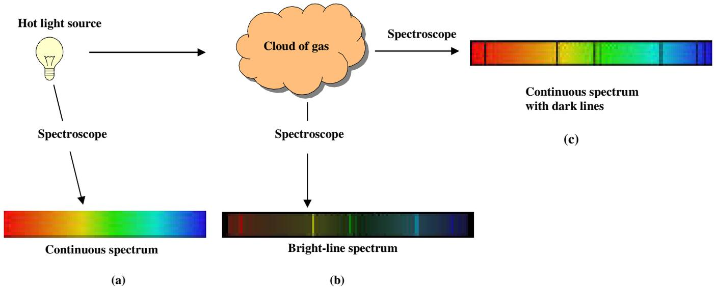
Fig.7.7: Diagrammatic representation of empirical rules for spectroscopic analysis of stellar spectra
