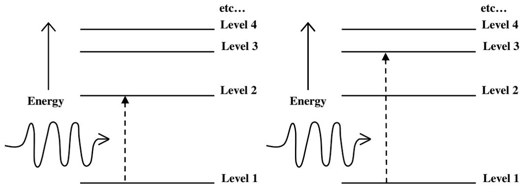
Fig.7.5: At high temperatures, electrons in hydrogen atoms get excited to various higher energy levels; transitions to levels 2 and 3 are shown here as examples
