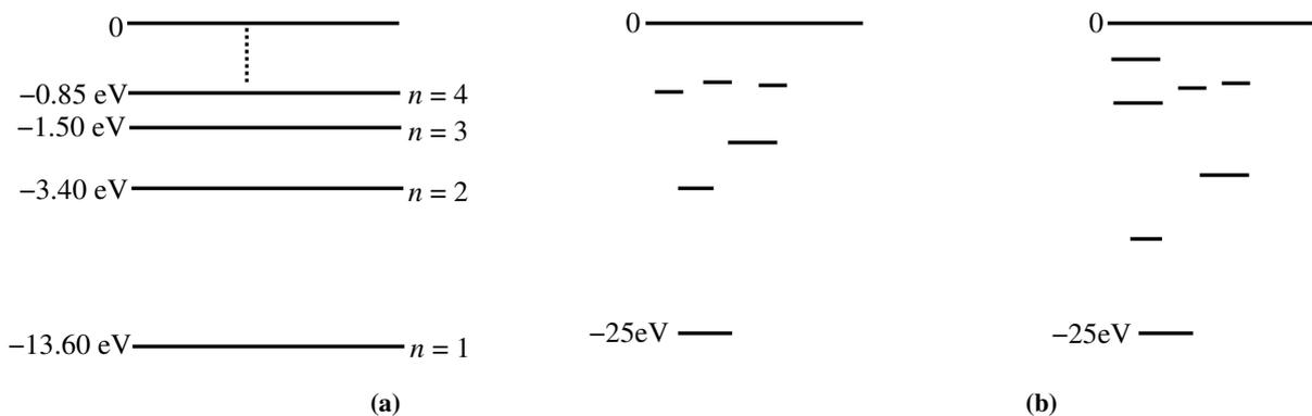
Fig.7.2: Energy level diagram of a) hydrogen atom; and b) helium atom
